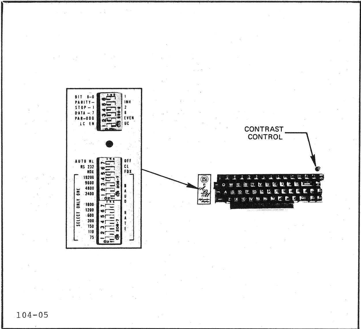
Figure 1-5. Front Panel Switch Locations
