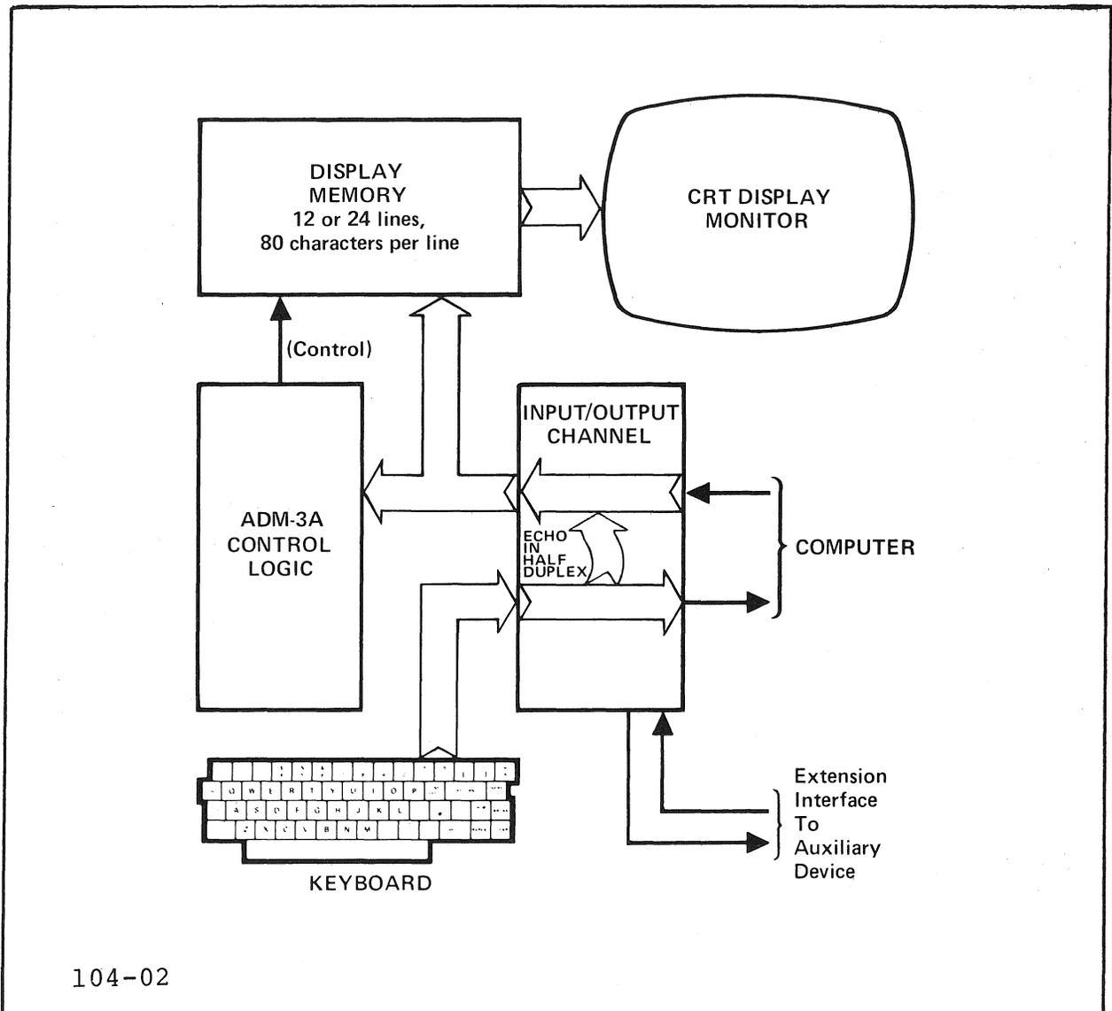
Figure 1-2. ADM-3A Data Flow Block Diagram
