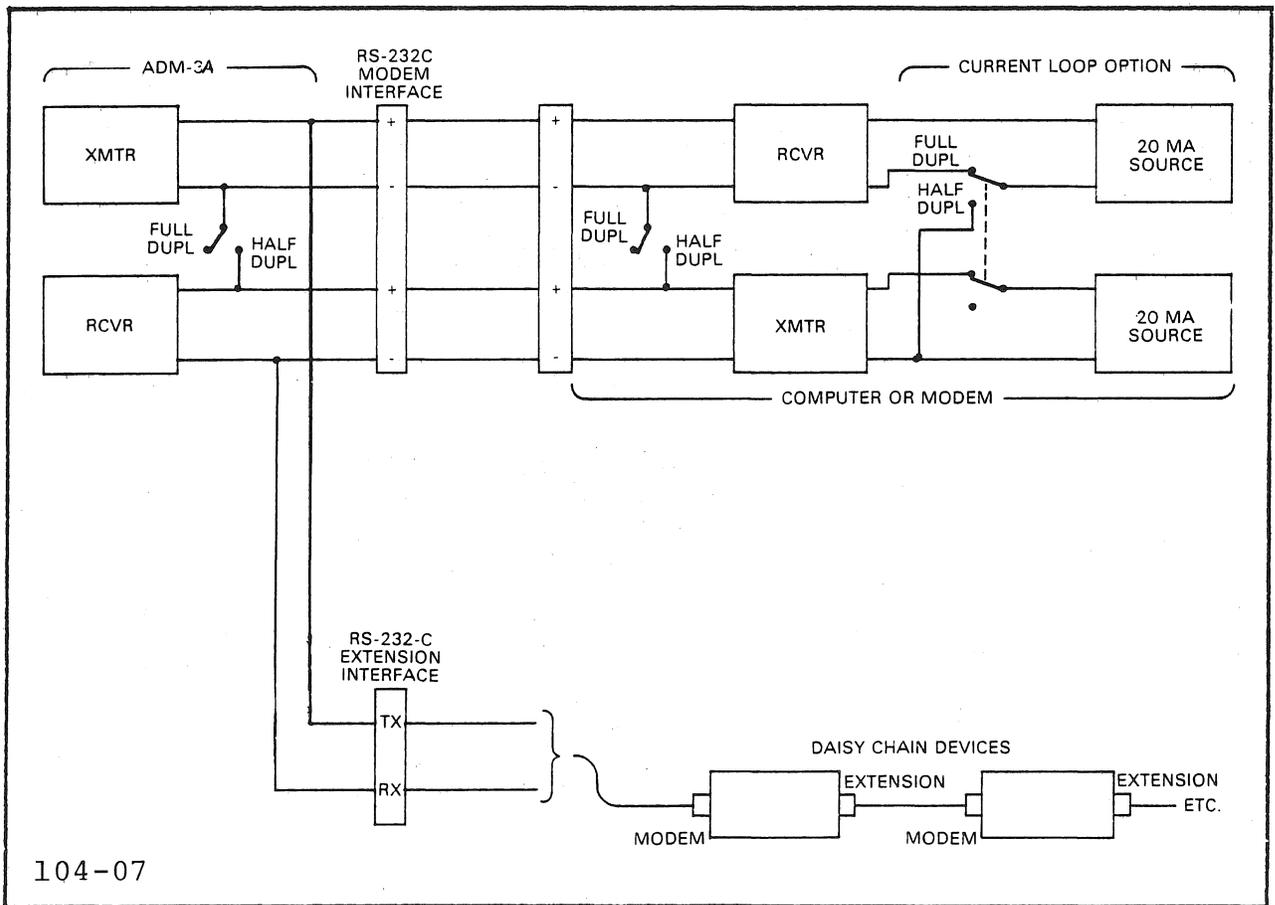
Figure 2-2. Typical ADM-3A Interfaces
