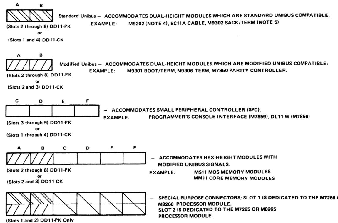
Figure 4-8 Module Placement
