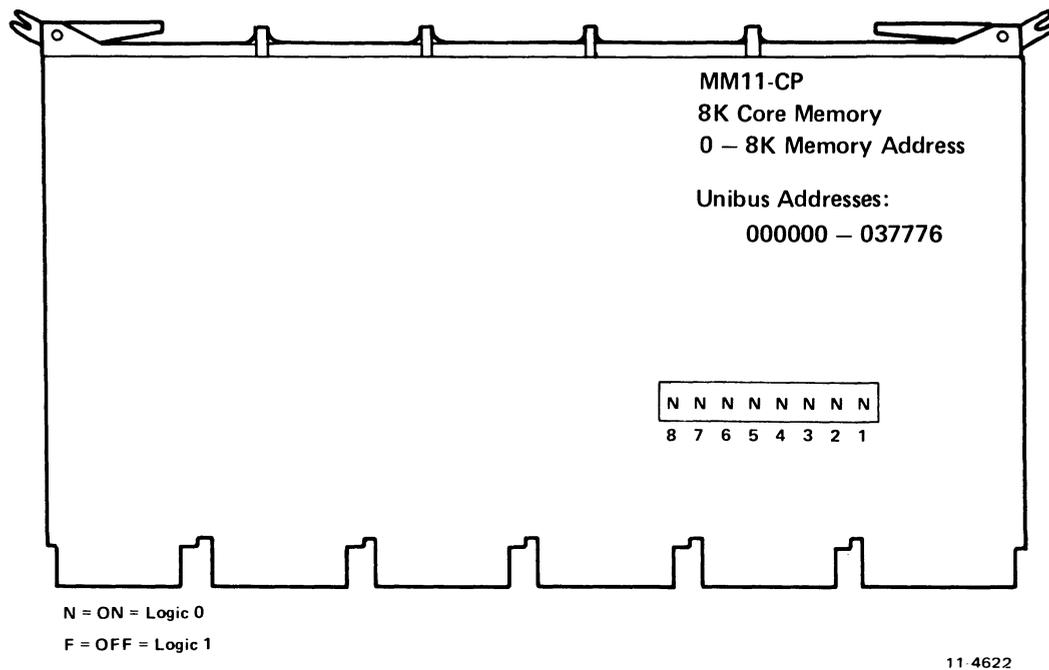
Figure 5-9 Typical Jumper Placement and Switch Settings of Modules
