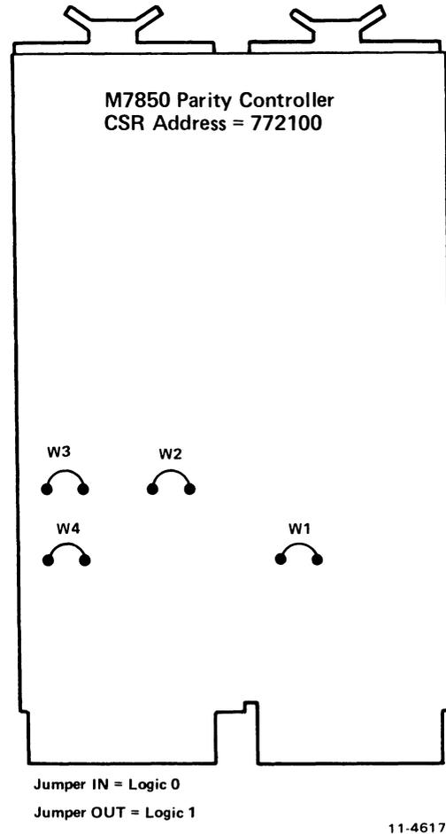
Figure 5-9 Typical Jumper Placement and Switch Settings of Modules
