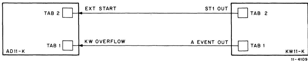
**Figure 2-6 Tab Connections**
