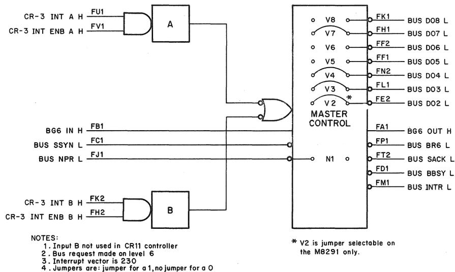
Figure 5-3 Interrupt Control Logic – Simplified Diagram
