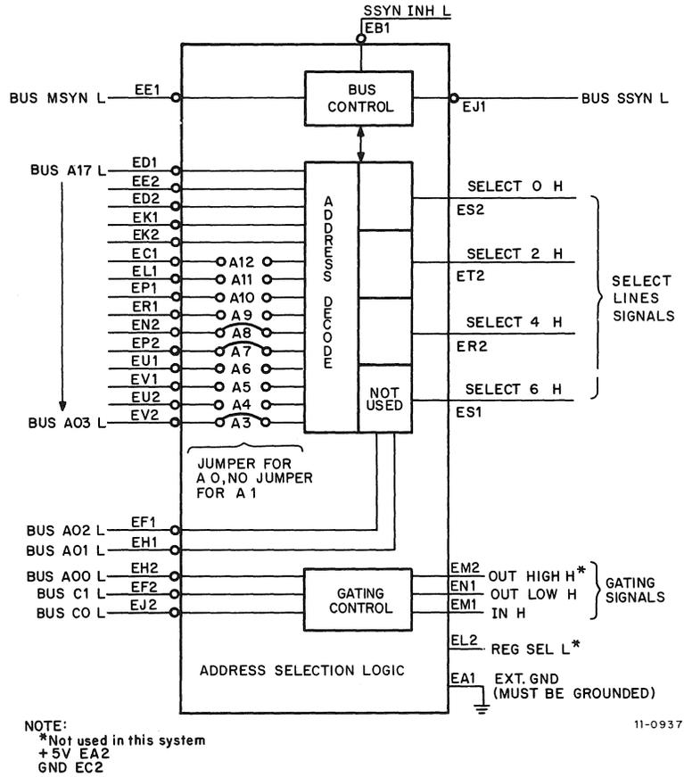
Figure 5-1 Address Selection Logic – Simplified Diagram
