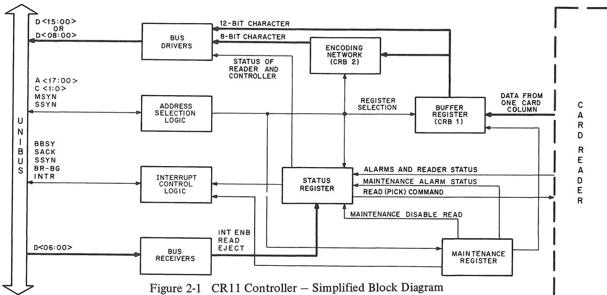
Figure 2-1 CR11 Controller – Simplified Block Diagram
