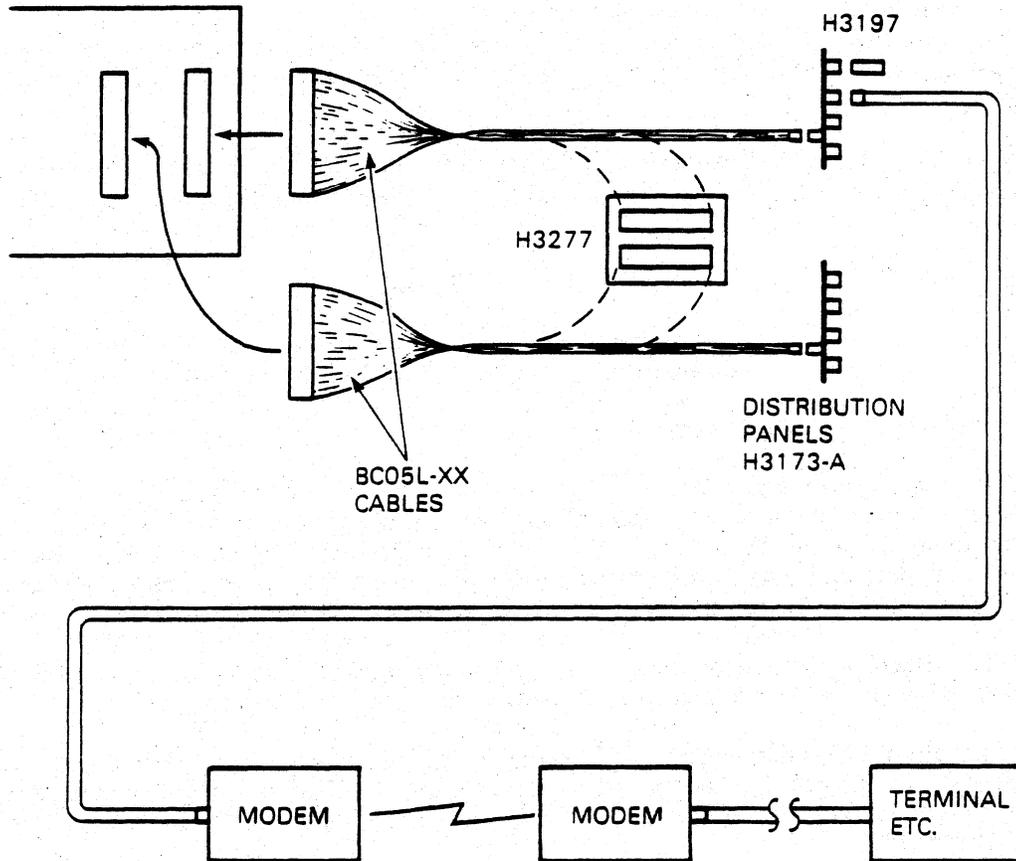
Figure 4-2 Using Loopback Connectors in EIA-232-D Installations
