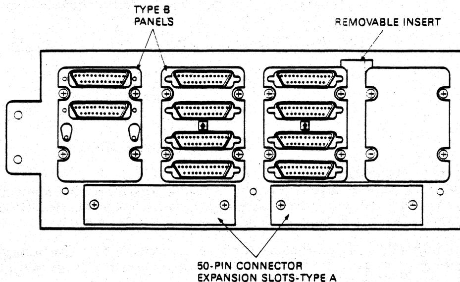
Figure 2-7 I/O Insert Panels and Adapter Plate (EIA-232-D)
