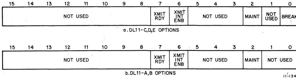
Figure 4-3 Transmitter Status Register (XCSR) – Bit Assignments
