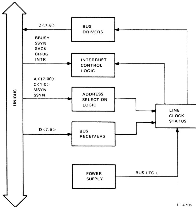
Figure 1-4 Line Clock Block Diagram
