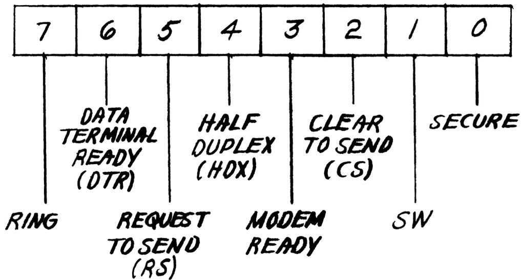
Figure 3-4 Modem Control Register Format
