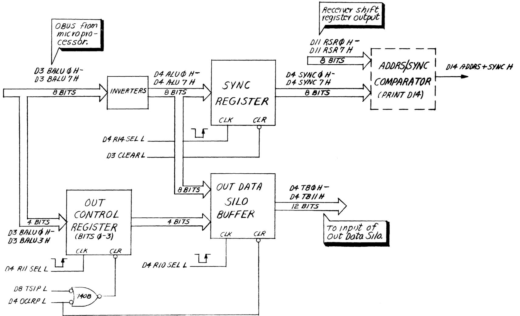
Figure 4-9 Block Diagram of OBUS and Associated Logic
