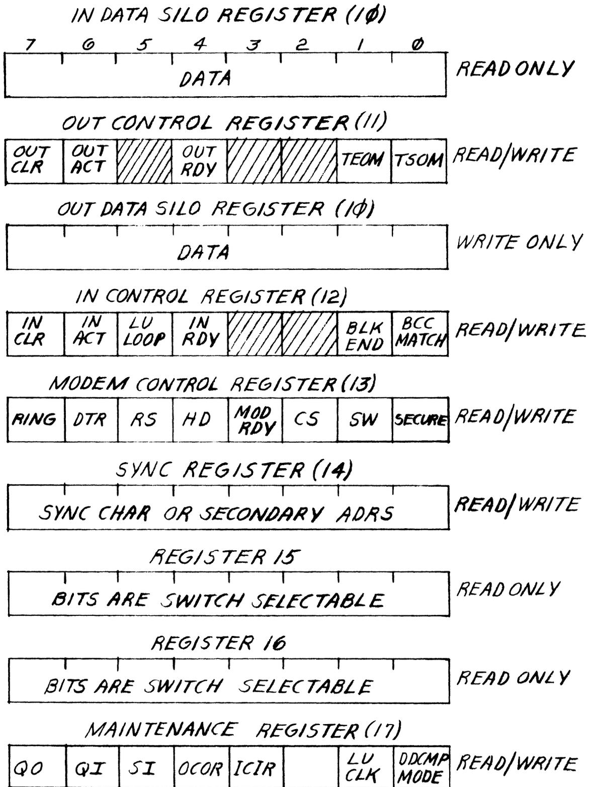
Figure 3-1 Line Unit Register Configurations and Bit Assignments
