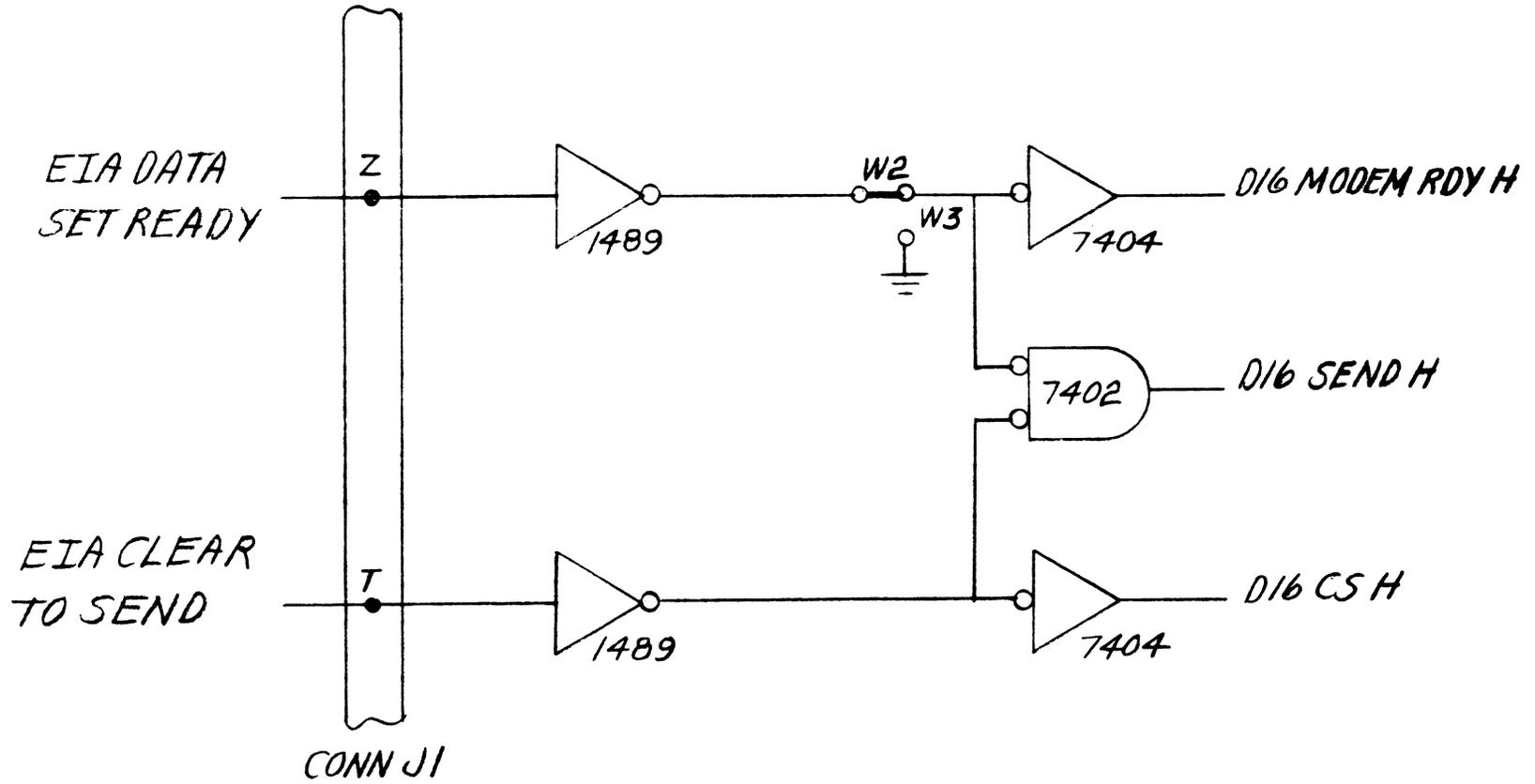
Figure 4-29 Conversion Logic for DSR
