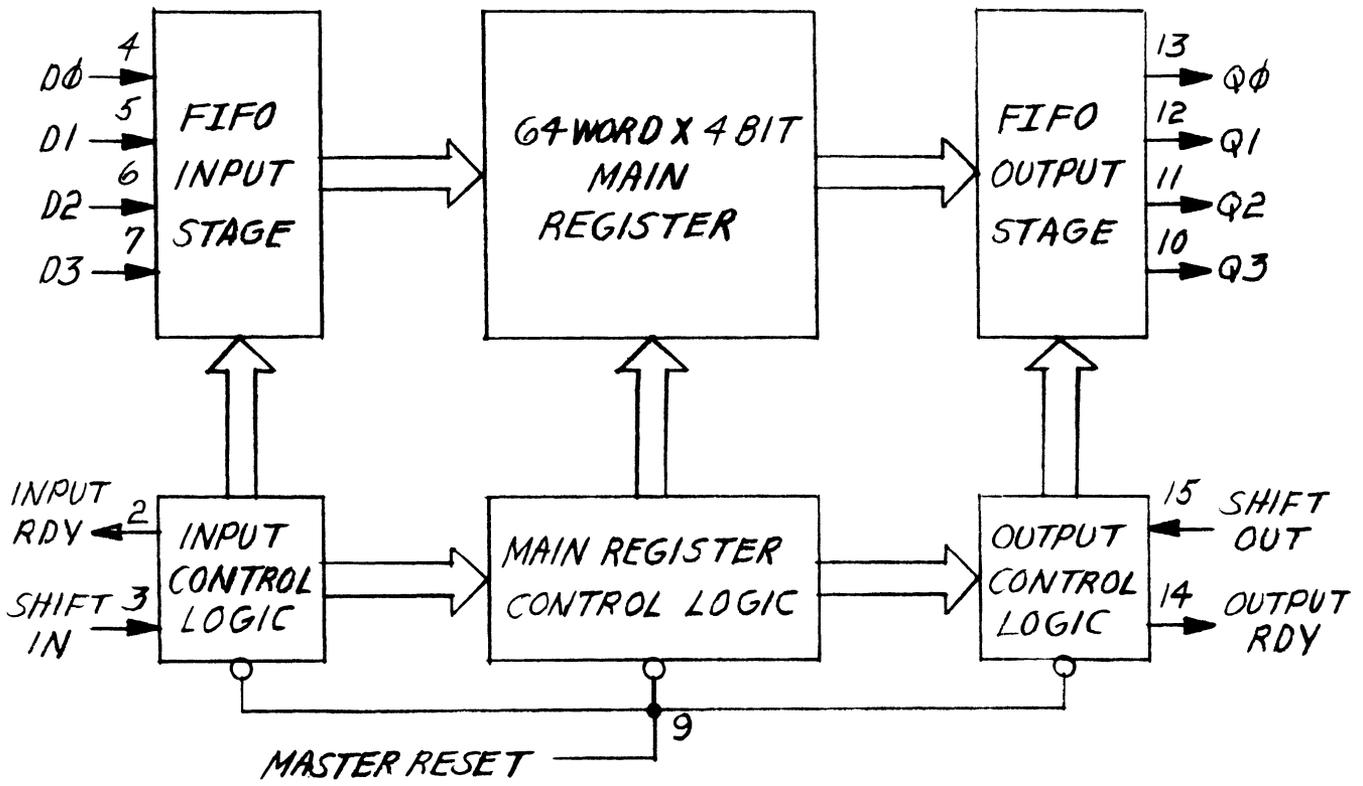
Figure 4-2 Logical Representation of 3341 FIFO
