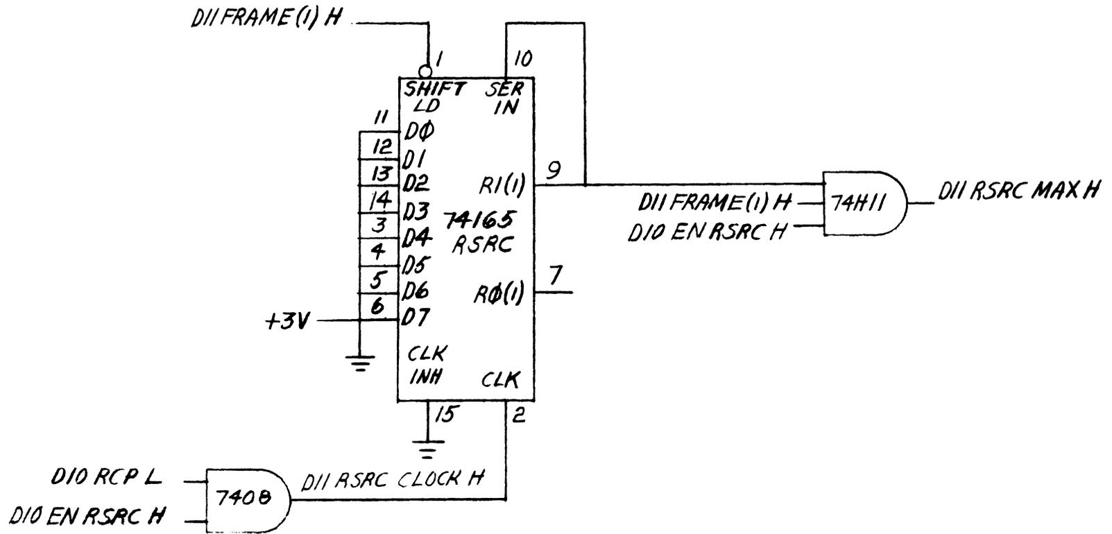
Figure 4-23 Receiver Shift Register Counter
