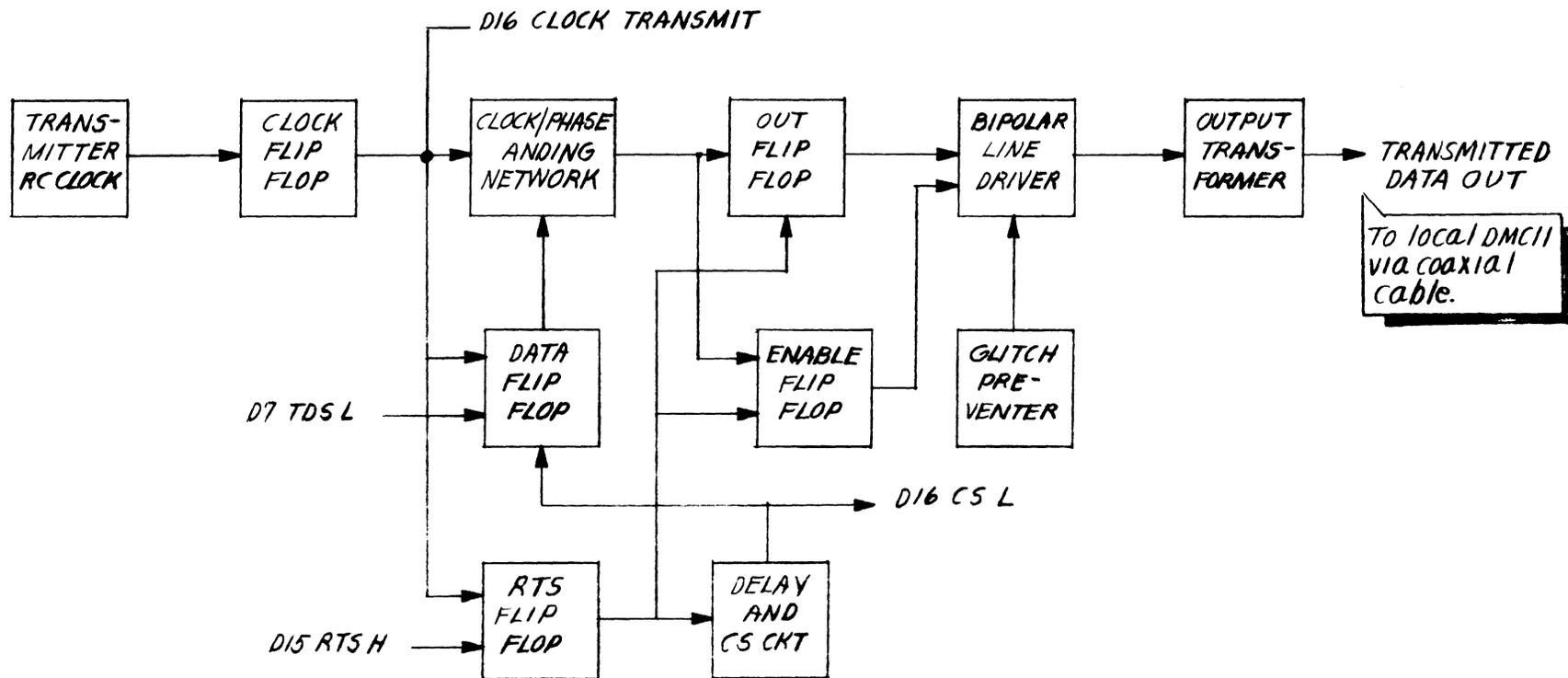
Figure 4-31 Simplified Block Diagram of Modem Transmitter
