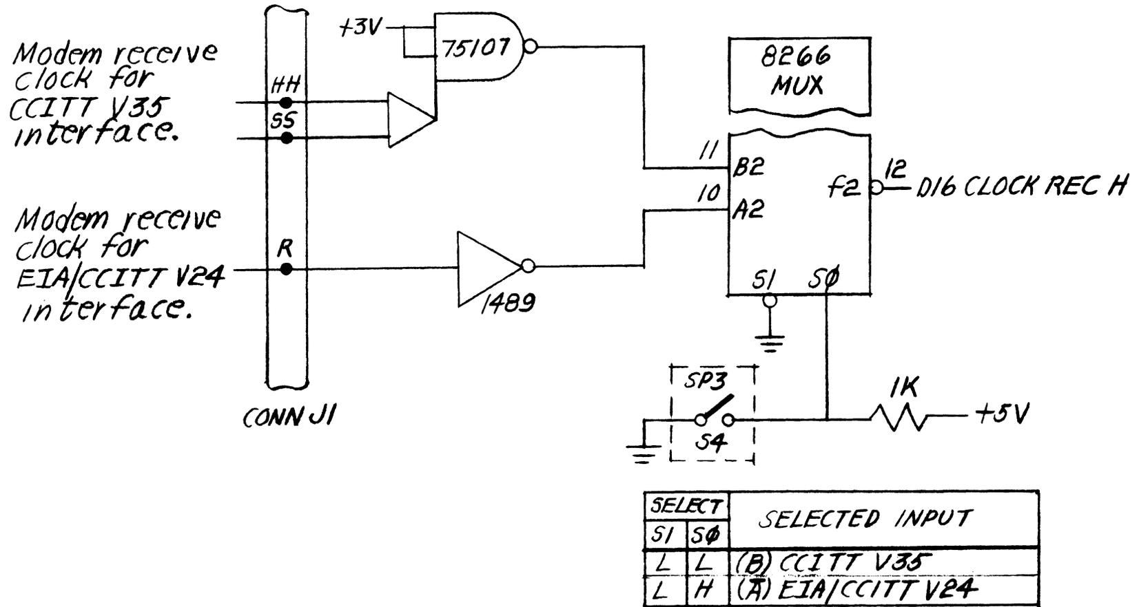
Figure 4-20 EIA Receiver Clock Conversion Logic
