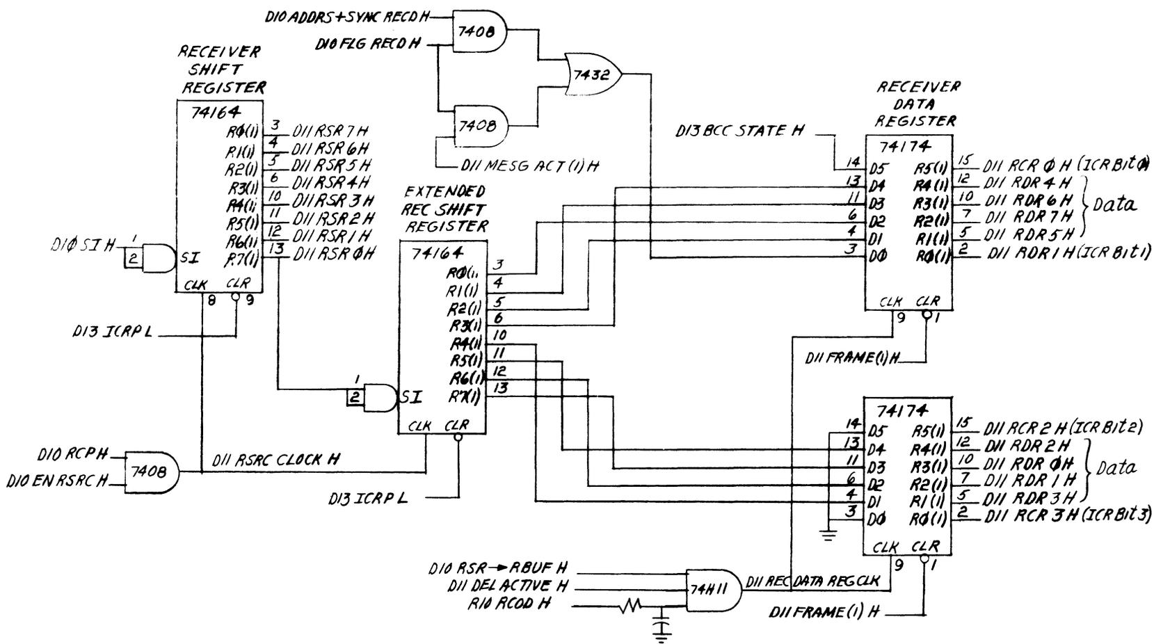
Figure 4-24 Receiver Shift Register and Data Buffer
