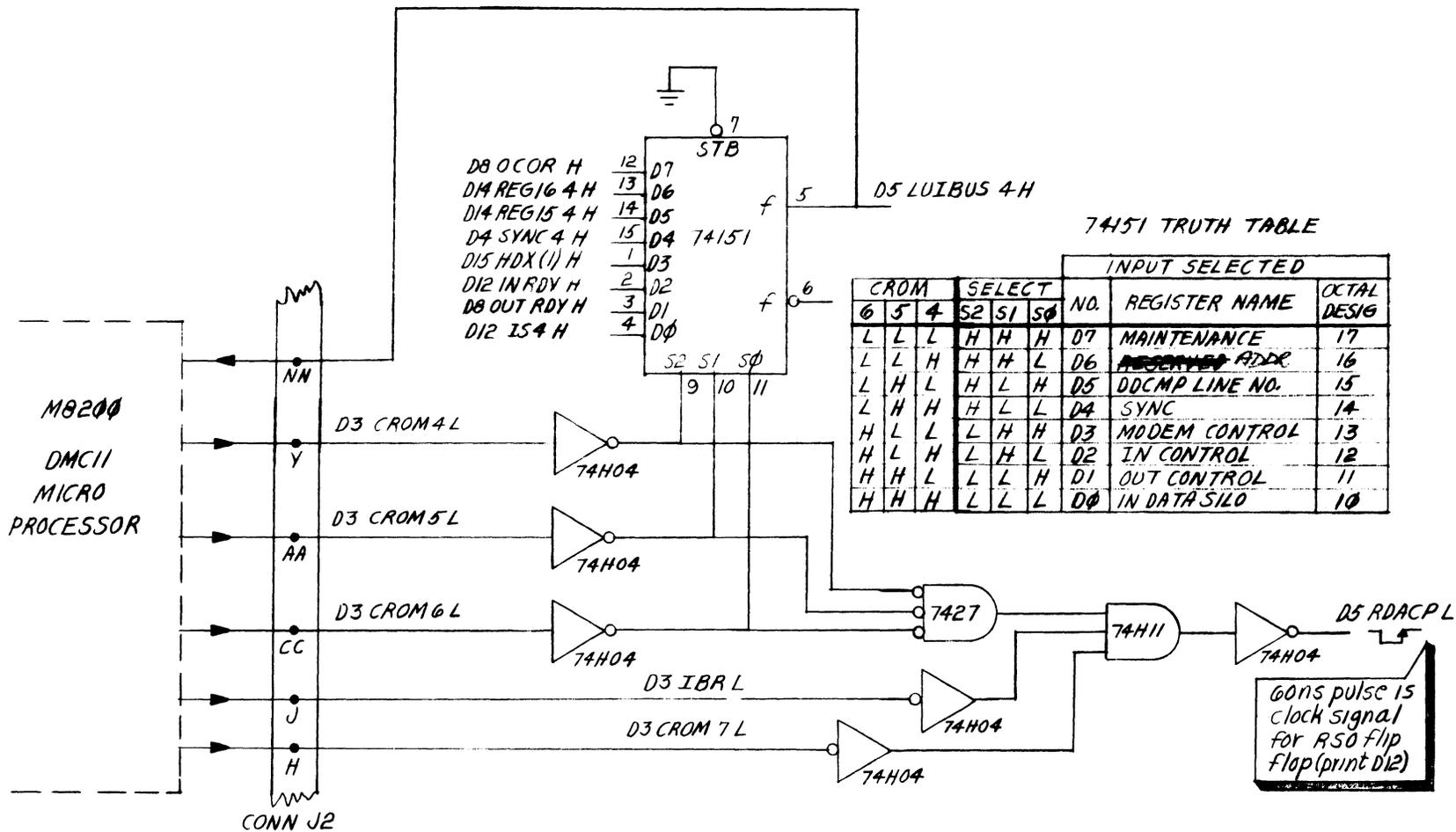
Figure 4-11 IBUS Control Logic (1-Bit Slice)
