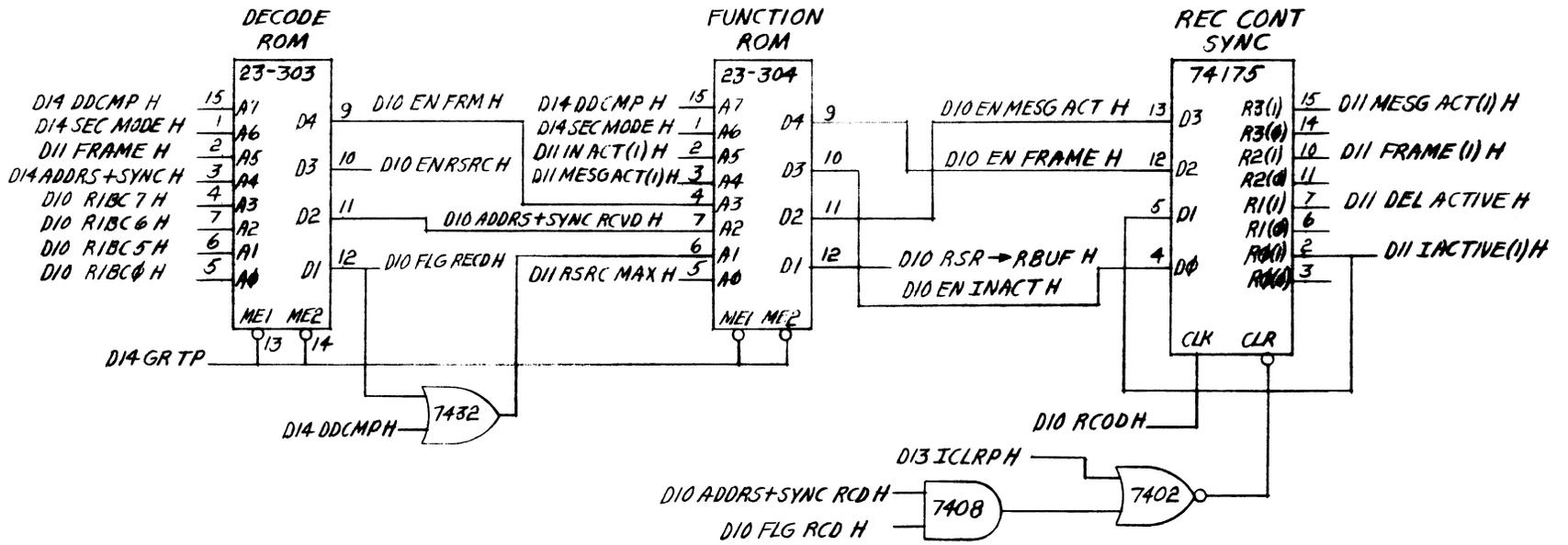
Figure 4-19 Receiver ROMs and Associated Logic
