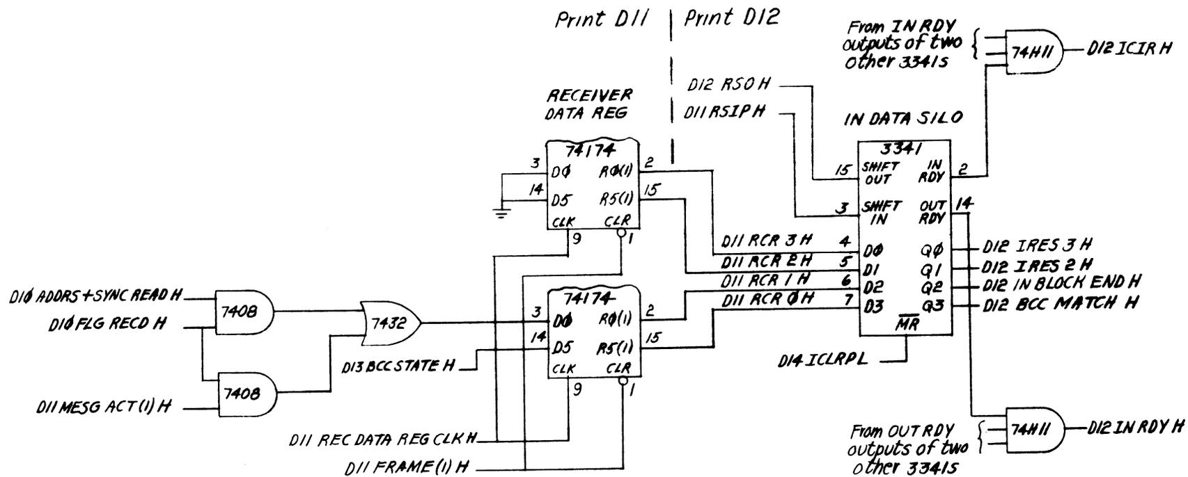
Figure 4-6 Logic for Input Control Register Bits 0-3
