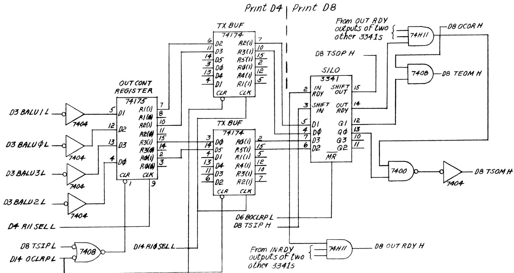
Figure 4-4 Logic for Output Control Register Bits 0-4
