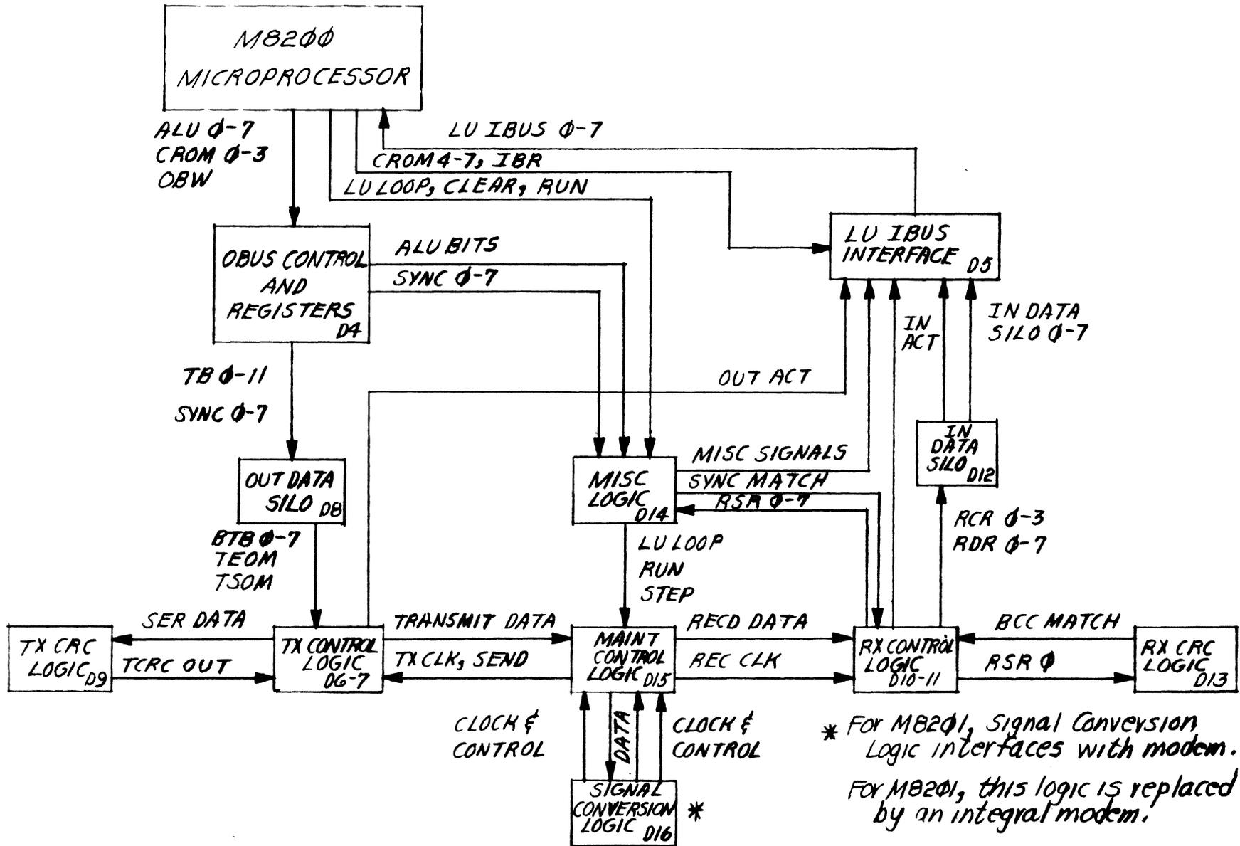
Figure 4-1 Line Unit Simplified Block Diagram
