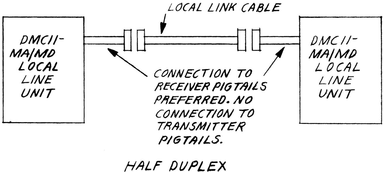
Figure 2-3 Full-Duplex/Half-Duplex Connections
