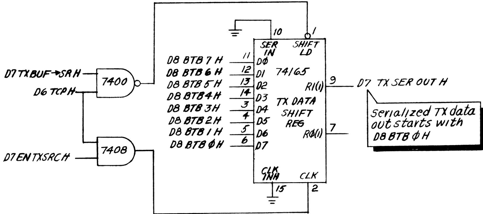
Figure 4-18 Transmitter Shift Register
