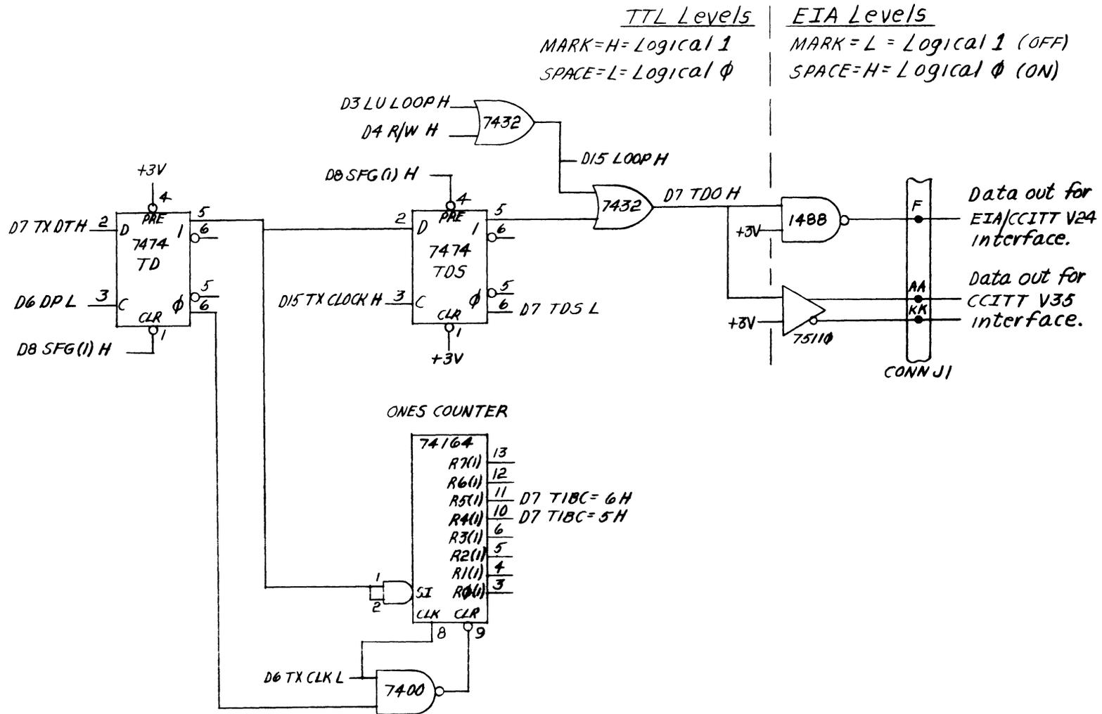
Figure 4-15 TD Flip-Flop and 1s Counter
