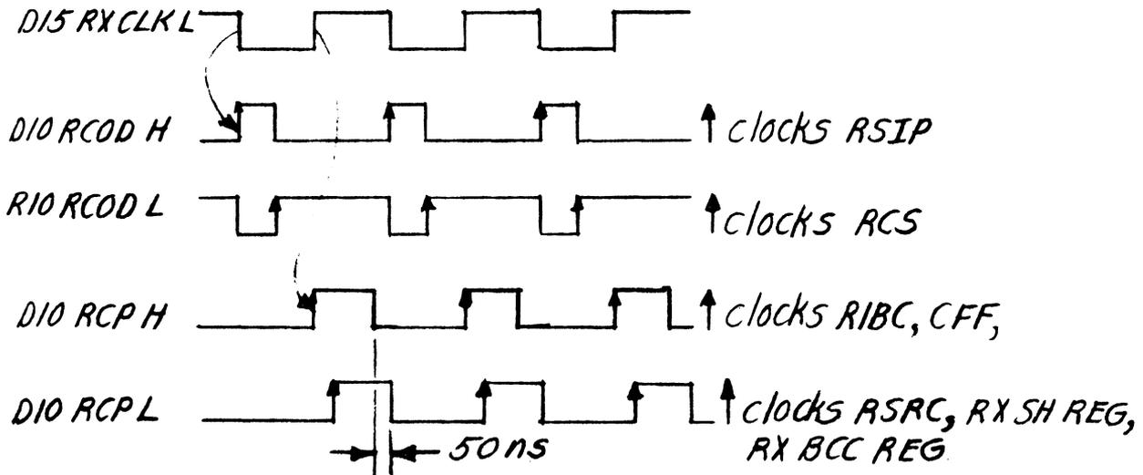
Figure 4-21 Receiver Clock Logic and Timing Diagram
