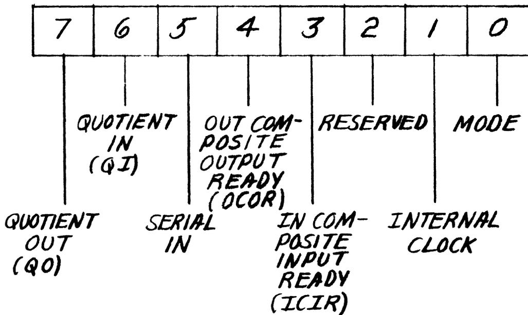
Figure 3-5 Maintenance Register Format
