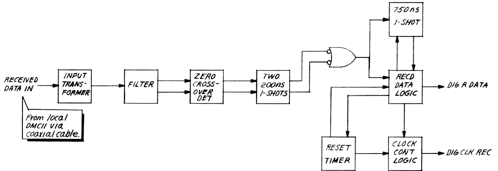
Figure 4-32 Simplified Block Diagram of Modem Receiver
