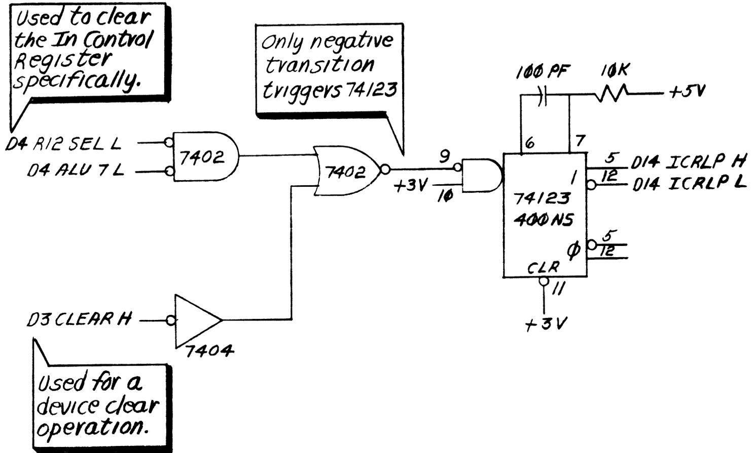
Figure 4-7 Logic for Input Control Register Bit 7
