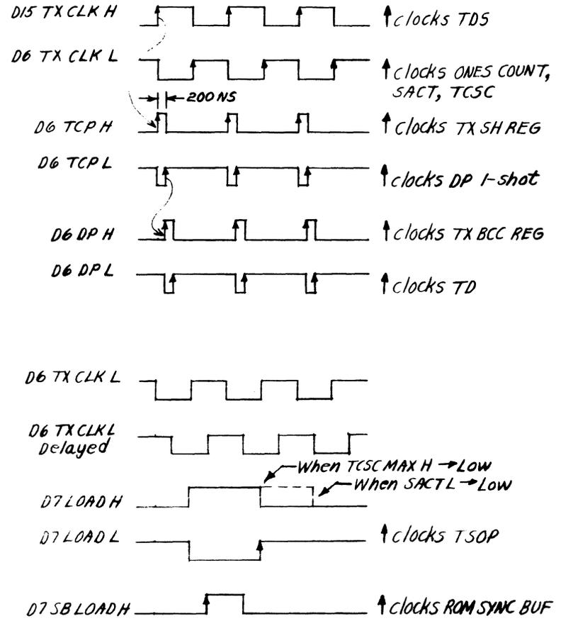
Figure 4-14 Transmitter Clock Logic and Timing Diagram
