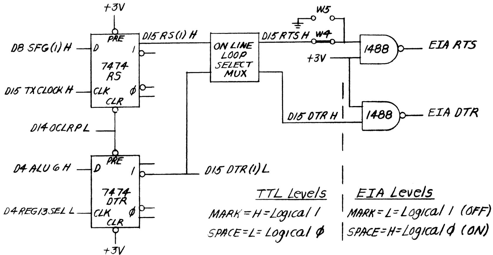
Figure 4-8 RTS and DTR Flip-Flops and Associated Drivers
