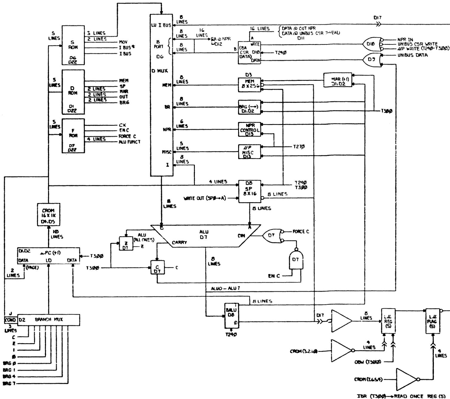
Figure 4-1 Microprocessor Block Diagram
