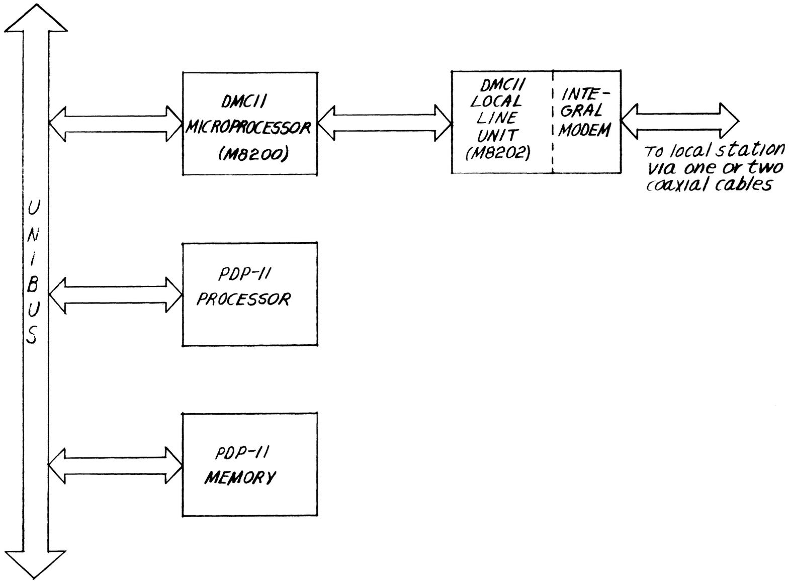
Figure 1-2 DMC11 Local Line Unit Interface
