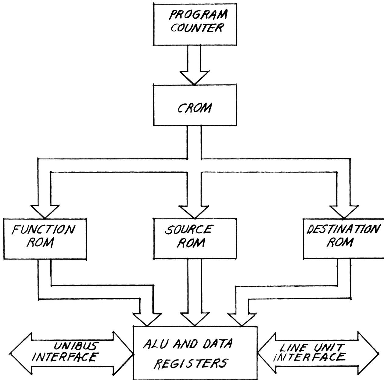
Figure 1-3 Microprocessor Simplified Block Diagram
