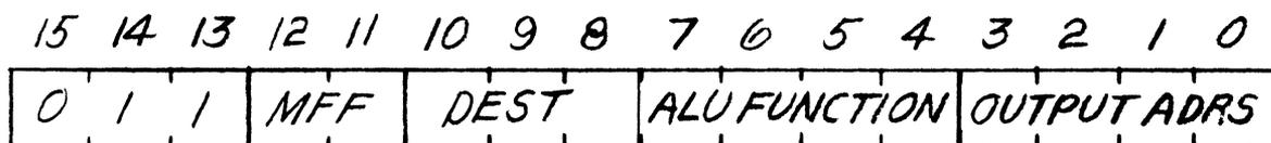
The operation of the MOVE BRG microinstruction is similar to the MOVE MEM with one exception. The two operands of this microinstruction are the contents of the BRG and the Scratch Pad memory. If the microinstruction specifies either the Scratch Pad memory or the BRG as the destination, then the respective source operand is destroyed by the delivery of the resultant operand.
