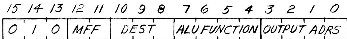
The MOVE MEM microinstruction performs either an arithmetic or logical operation on two designated operands and deposits the result operand into the specified destination address. One of the two operands is from MEM while the second is from the Scratch Pad memory. The specific location within the SCRATCH PAD memory
