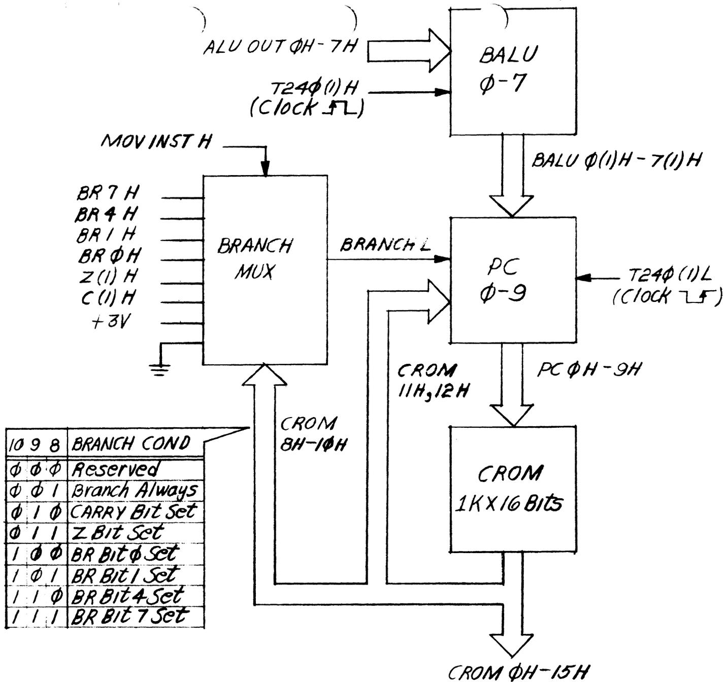
Figure 4-5 Block Diagram of Program Counter Control Logic
