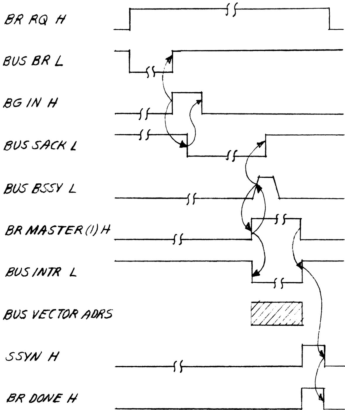
Figure 4-19 Interrupt Timing Diagram
