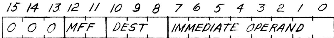
The operand, microinstruction bits 0-7, is moved to the destination as specified by microinstruction bits 8-10.
