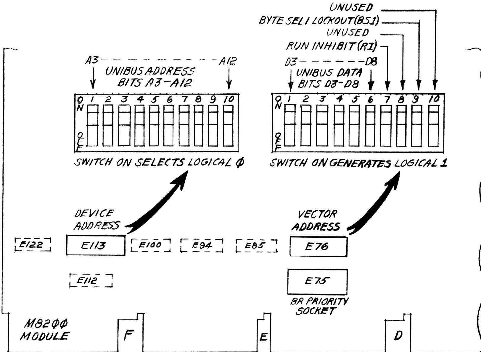
Figure 2-1 Microprocessor Device and Vector Address Switches
