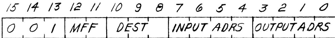
The operation code specifies the I BUS as the source operand. However, because the IBUS is a block of sixteen 8-bit words additional address information must be provided by the INPUT
