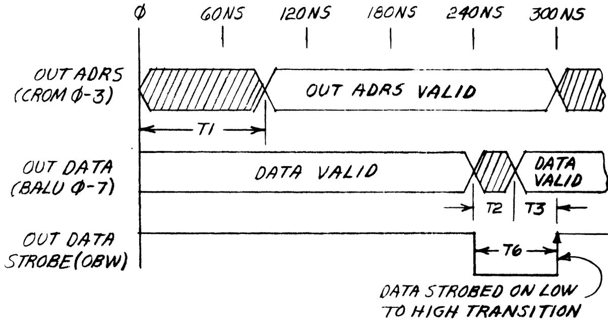
Figure 4-20 Typical Output Bus Timing
