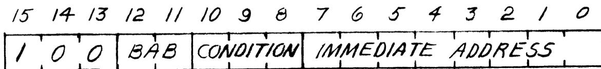
The microprogram branches if the condition specified by microinstruction bits 8-10 is met. The ten bit branch address
