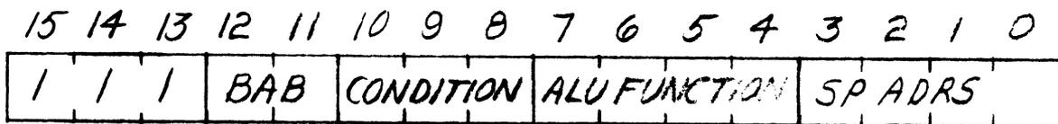
With this microinstruction, the contents of the BRG and a Scratch Pad memory location are operated on to generate the partial branch address. Bits 0-3 specify the Scratch Pad memory location and bits 4-7 define the ALU FUNCTION to perform on the two operands.
