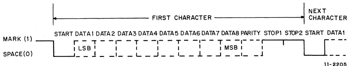
Figure C-1 Format of Typical Input/Output Serial Character
