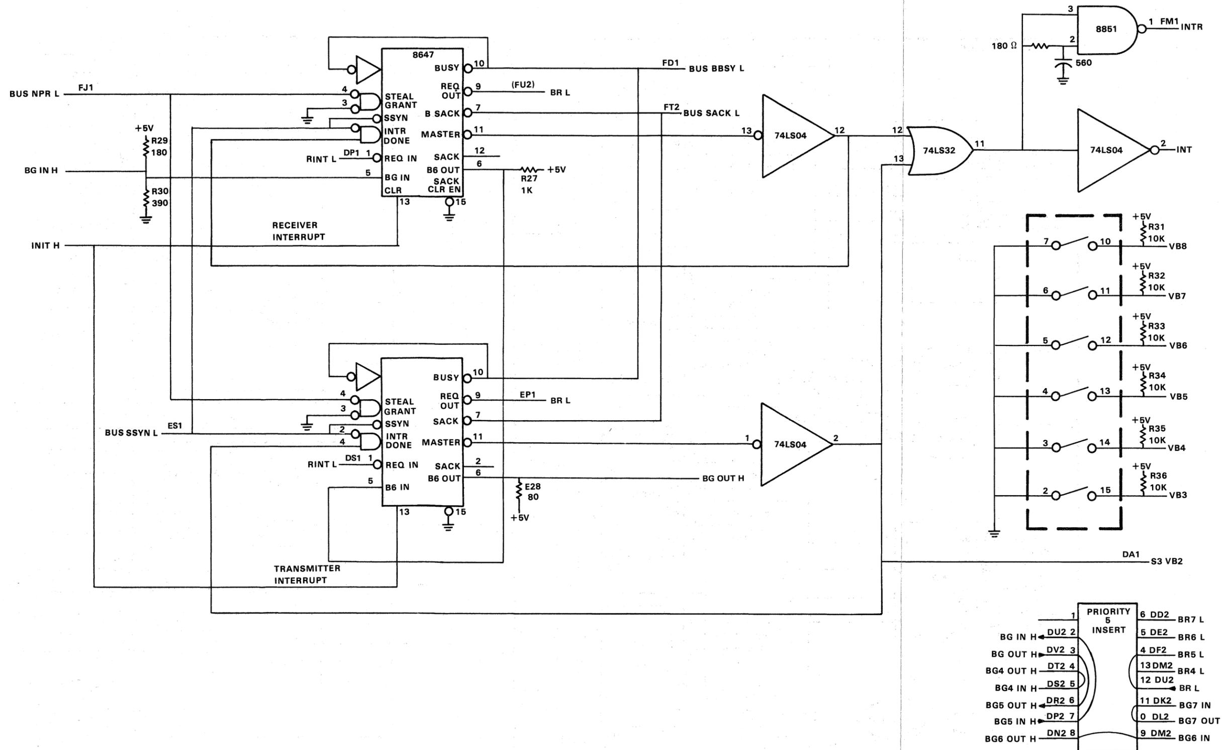
Figure 4-10 Interrupt Control Logic
