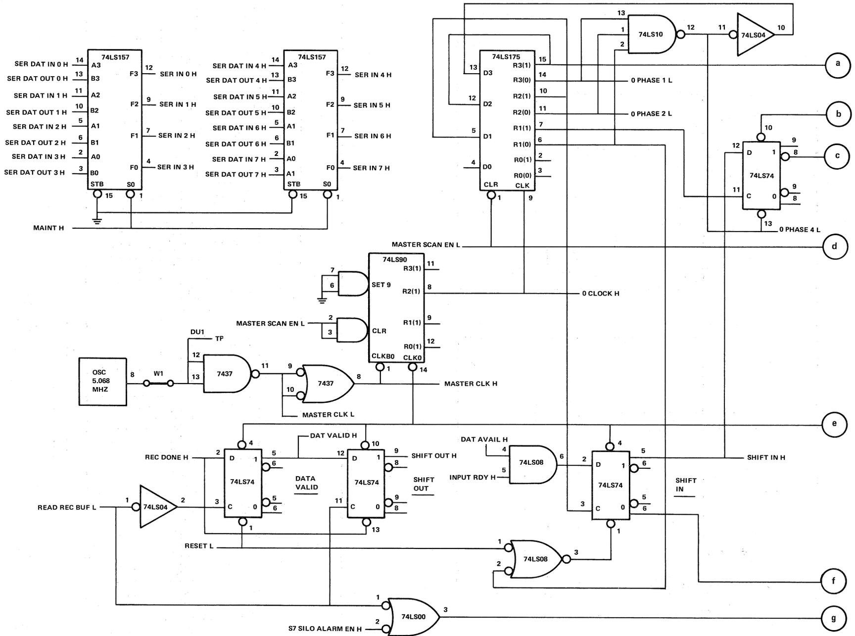
Figure 4-12 Receiver Control Logic
