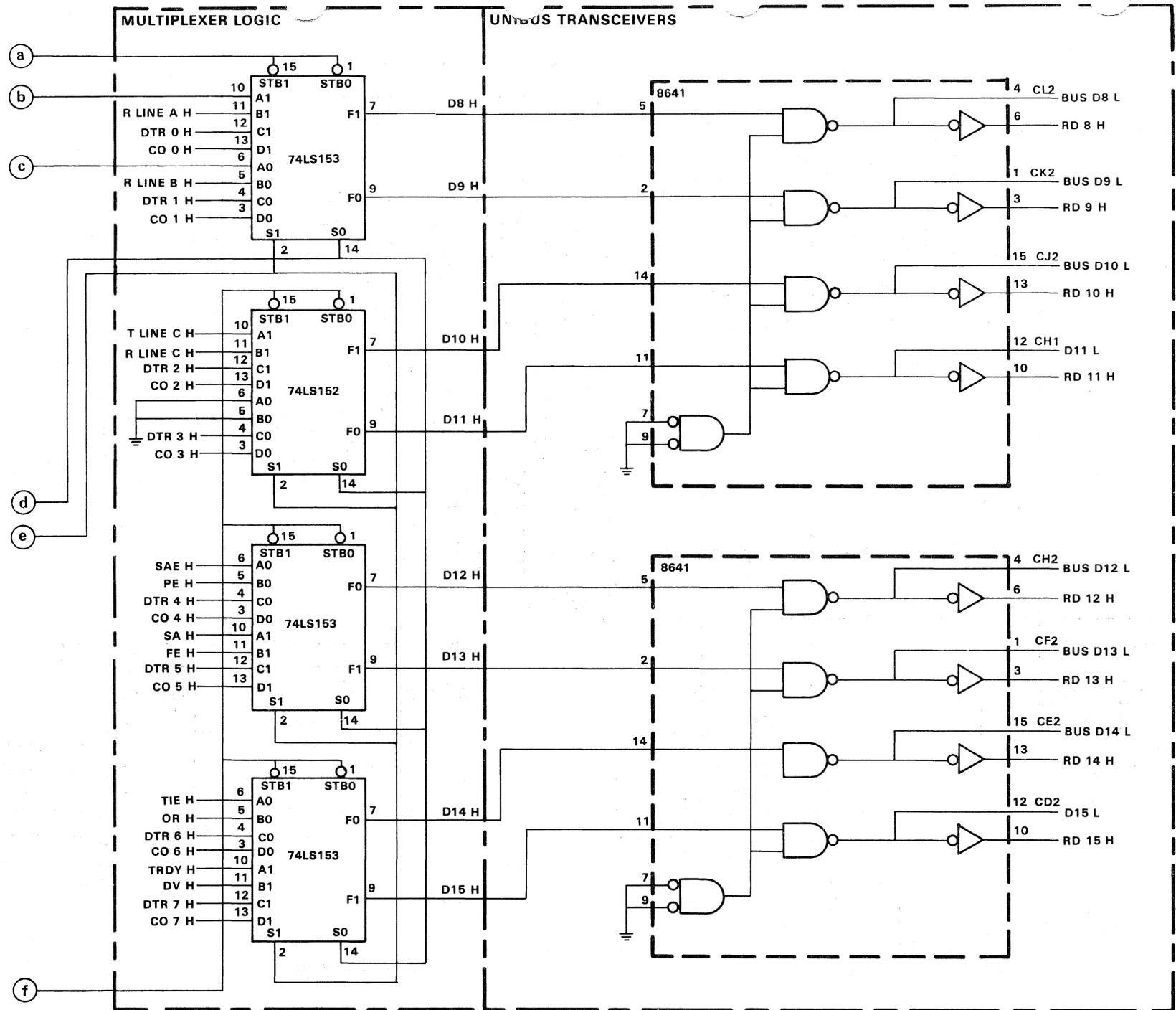
Figure 4-11 Unibus Data Flow
