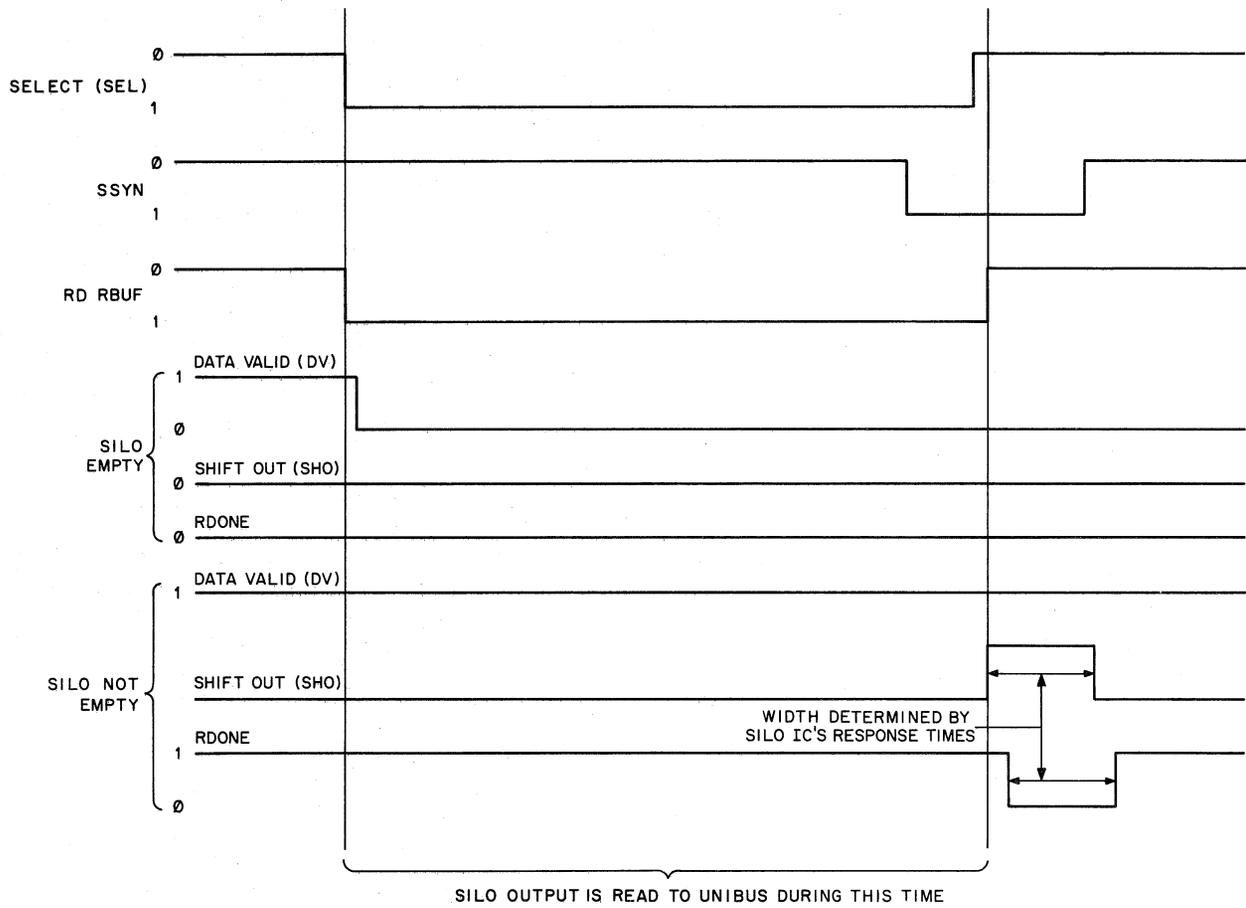
Figure 4-14 Silo Character Shift Out Timing Diagram
