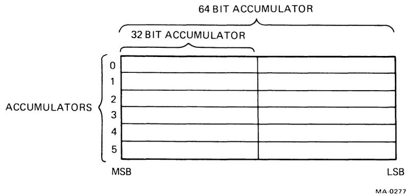
Figure 5-1 Floating-Point Accumulators
