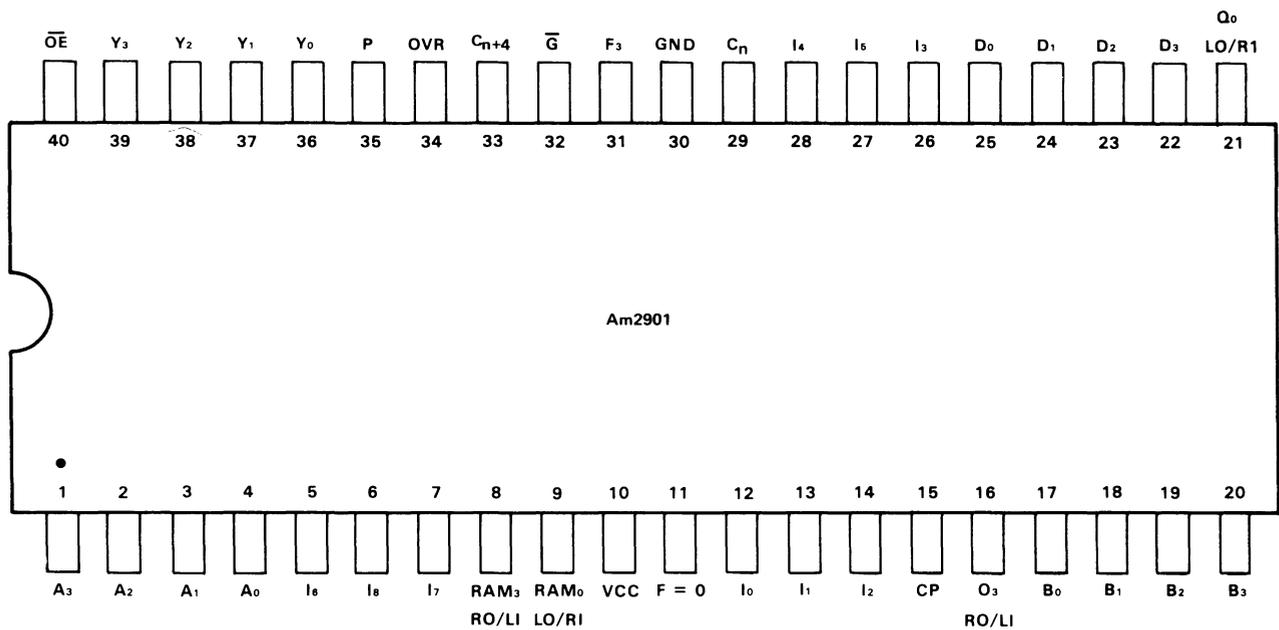
NOTE: PIN 1 IS MARKED FOR ORIENTATION.
