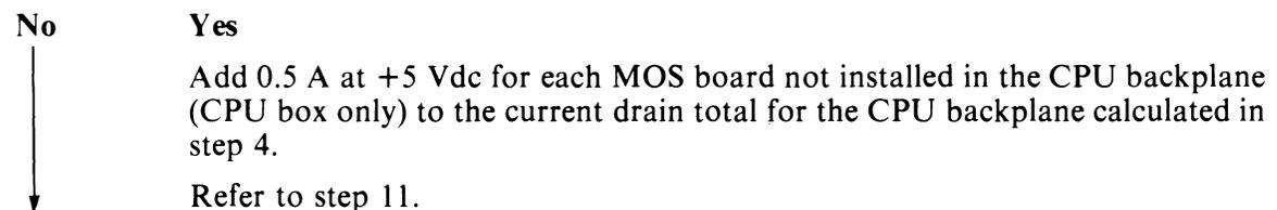
11. Is the CPU backplane current drain less than 25 A at +5 Vdc?
