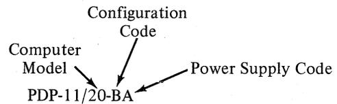
2. Examples are: PDP-11/20-BA is basic system with Teletype, table-top model, 115V version
