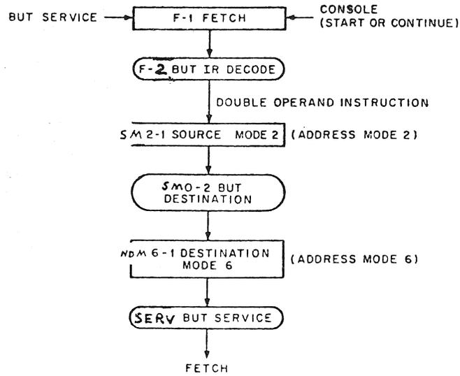
Figure 34 CMP #15, CHAR (022767), Simplified Flow Diagram
