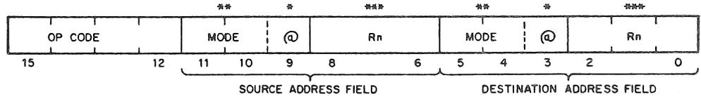
\* = DIRECT/DEFERRED BIT FOR SOURCE AND DESTINATION ADDRESS
