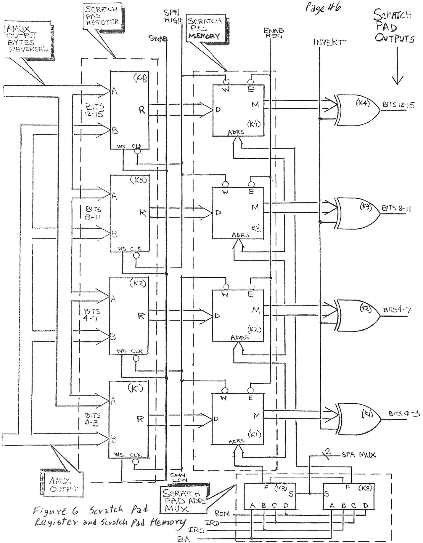
Figure 6 Scratch Pad Register and Scratch Pad Memory
