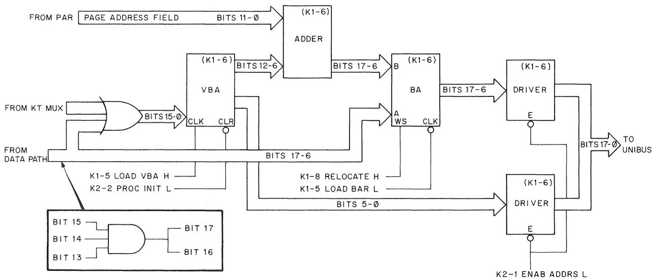
Figure 4-18 Unibus Address Logic Block Diagram
