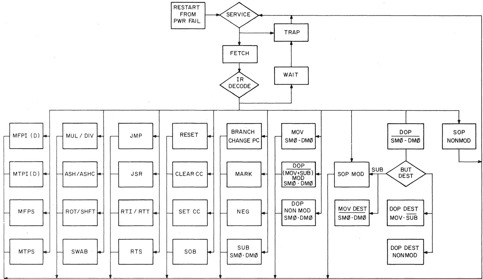
Figure 5-1 KD11-E Simplified Flow Diagram
