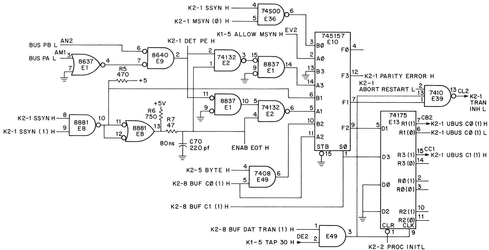
Figure 4-22 Data Transfer Multiplexer
