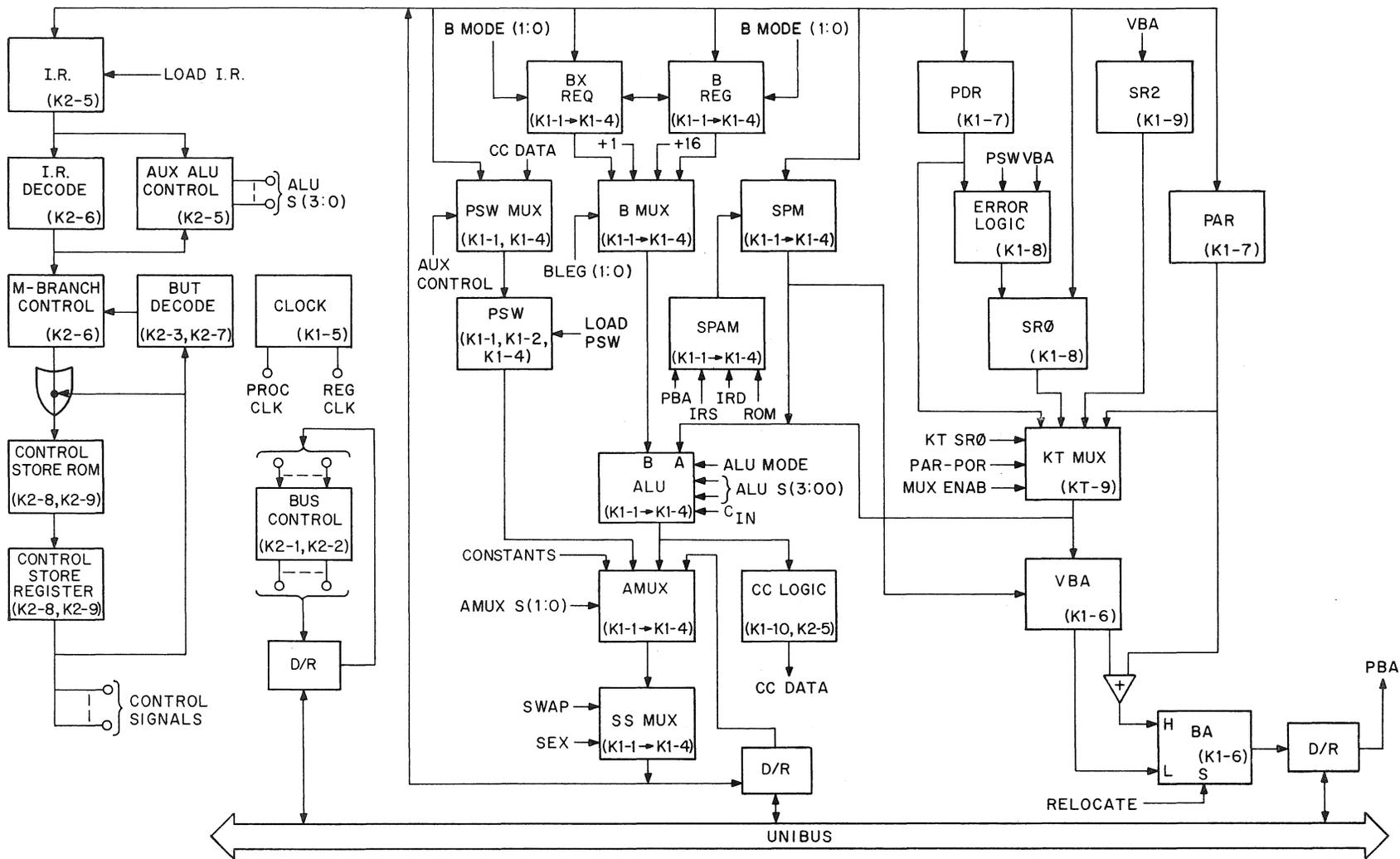
Figure 4-1 KD11-E Block Diagram
