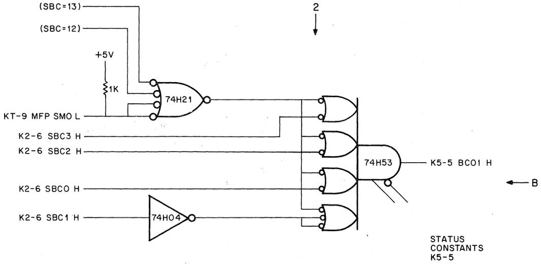
Figure 2-13 KT-9 MFP SM0L Hook In KD11-A
