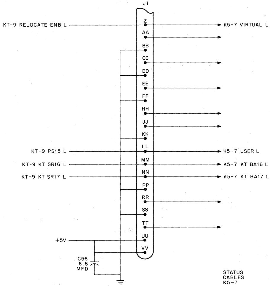
Figure 2-14 Console MM Enable Hooks In KD11-A
