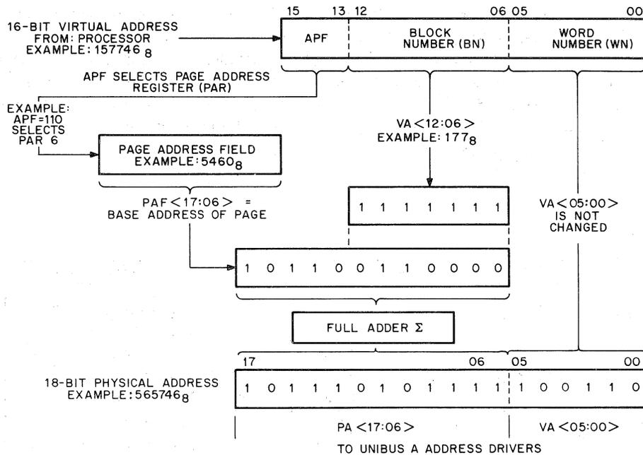
Figure 3-3 Construction of an 18-Bit Physical Address
