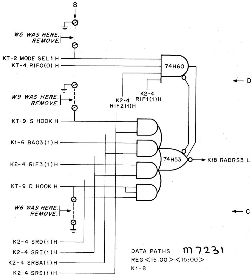
Figure 2-2 KD11-A Wiring Change No. 2
