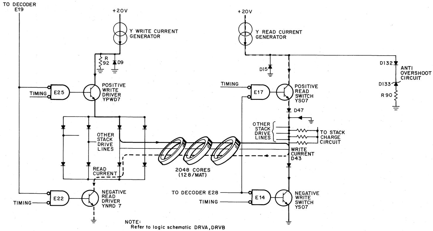
Figure 3-5 Typical Y Line Read/Write Switches and Drivers
