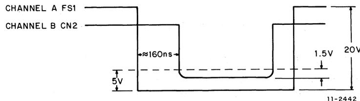
Figure 5-3 Sense Strobe Delay Waveform
