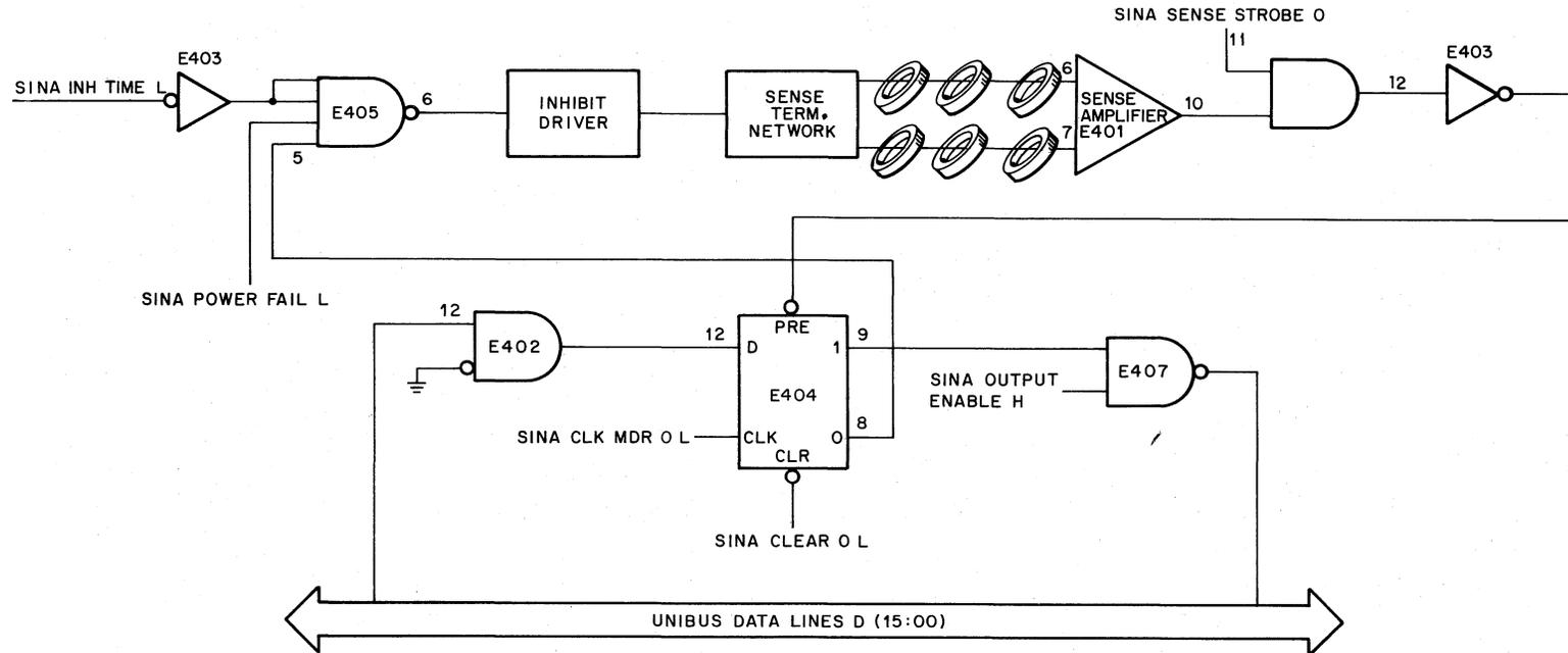
Figure 3-6 Interconnection of Unibus, Data Register, Sense Amplifier and Inhibit Driver
