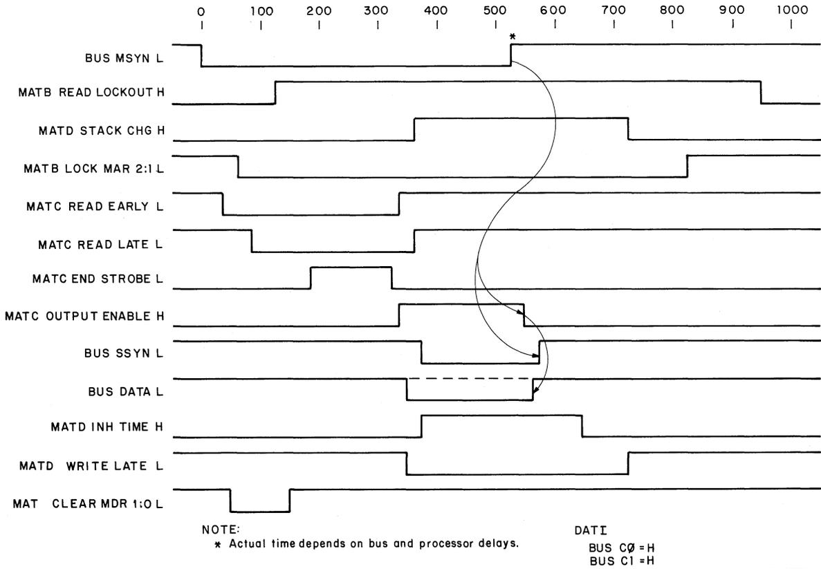
Figure 2-5 DATI Mode Timing Diagram
