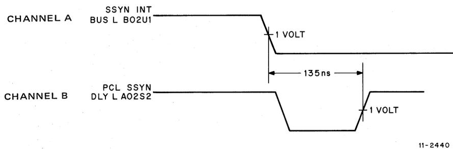
Figure 5-4 SSYN DLY L Timing Waveform
