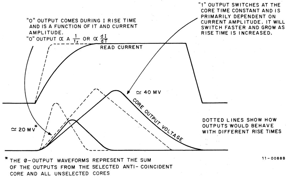
Figure 3-3 Core Current/Voltage Output Relationship
