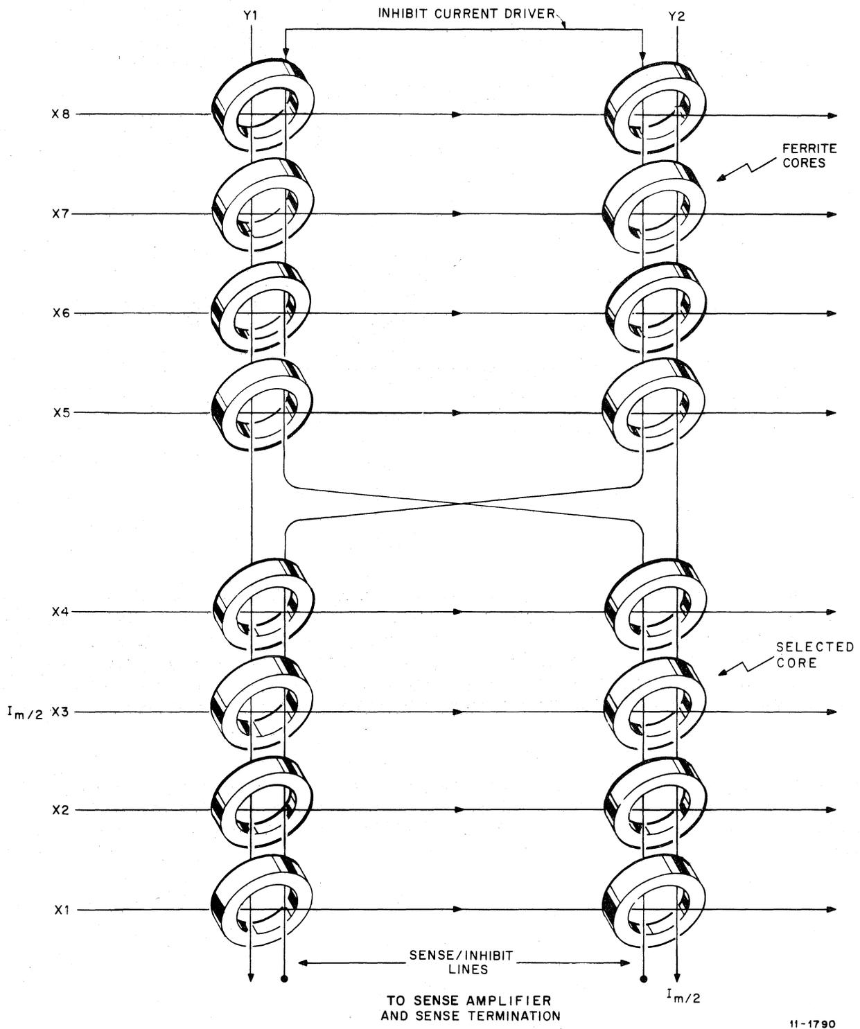
Figure 3-4 3-Wire Configuration
