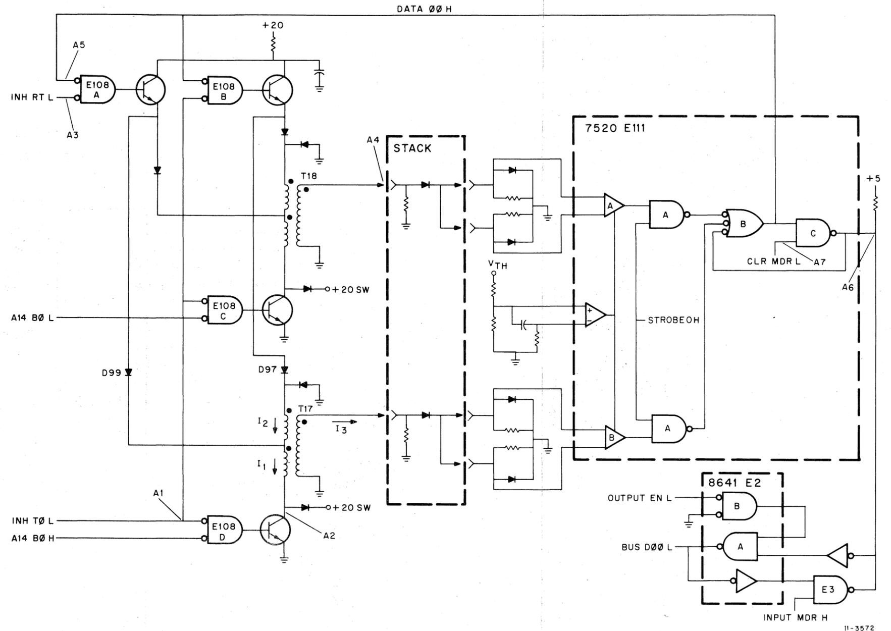
Figure 4-5 Waveform Key A (Sense/Inhibit Circuit)
