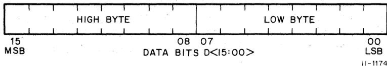
Each byte is addressable and has its own address location; low bytes are even numbered – high bytes are odd numbered. Words are addressed at even-numbered locations only; the high (odd) byte is automatically included.
