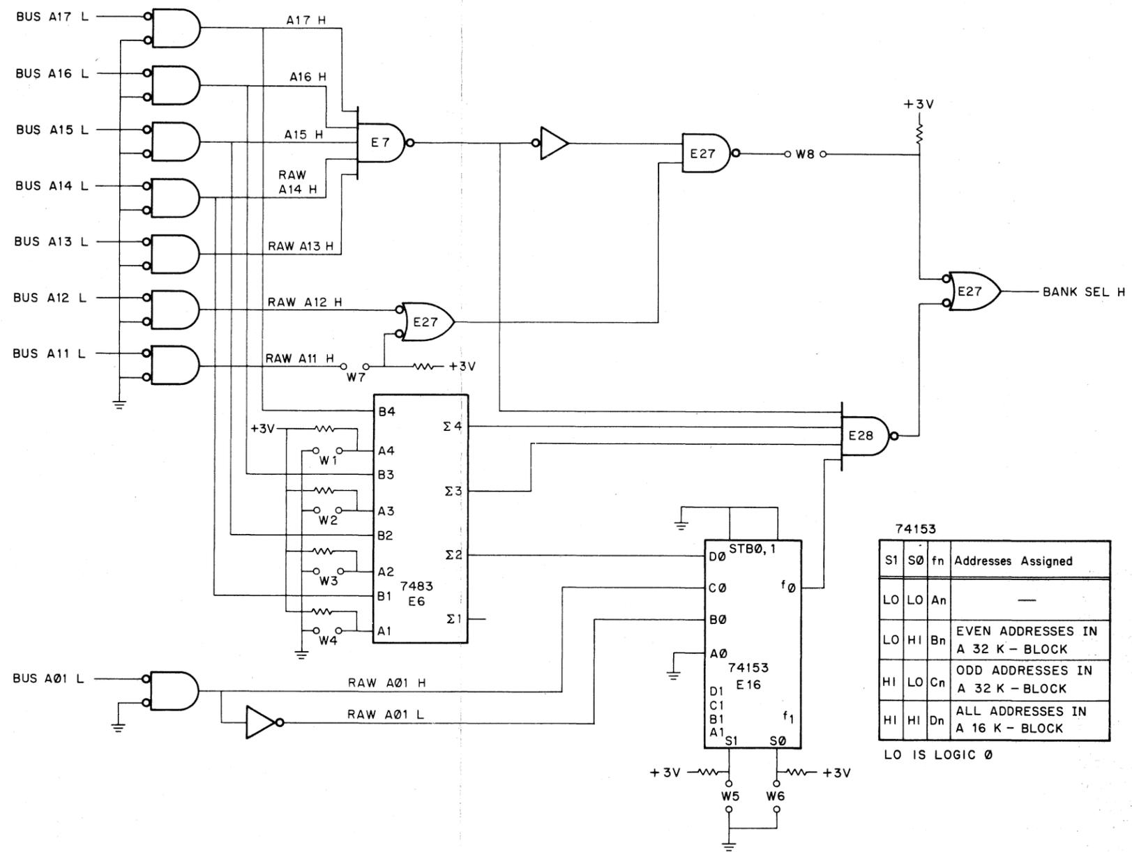
Figure 3-12 Address Decoding Logic
