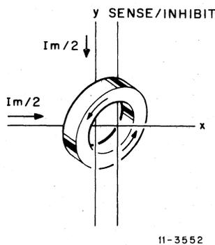
Figure 3-1 Core Windings
