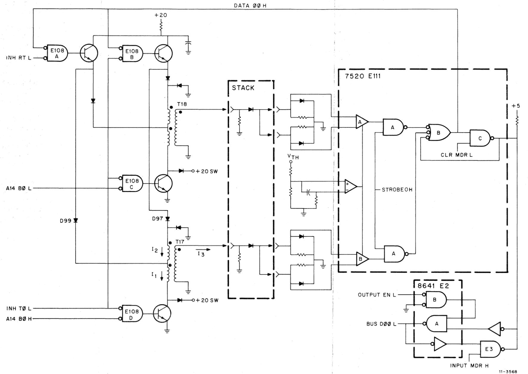
Figure 3-23 Sense/Inhibit Circuit (Bit 00)
