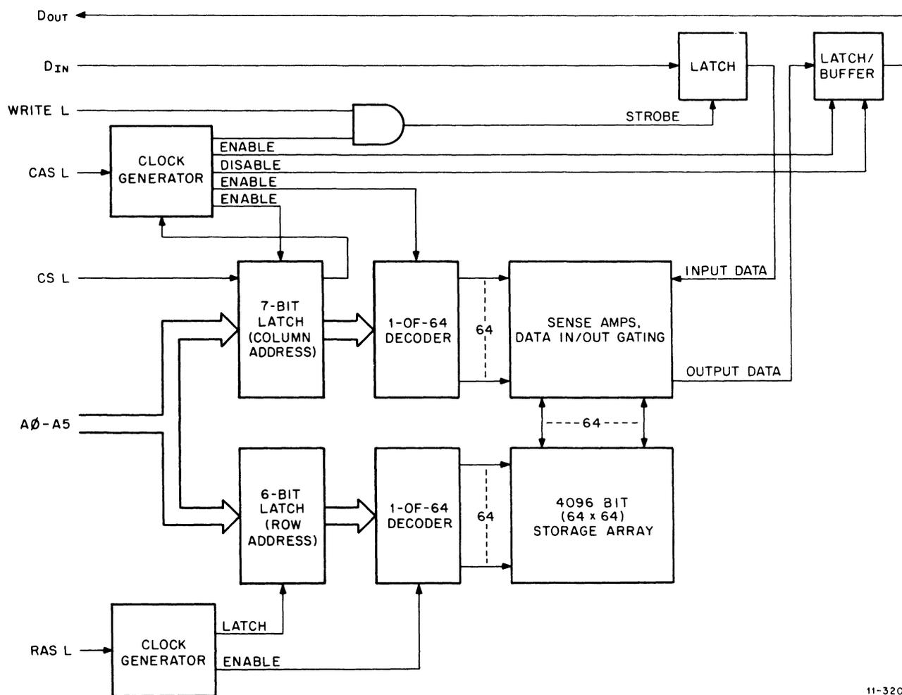
Figure 3-2 (4096 x 1) Bit MOS Chip, Block Diagram
