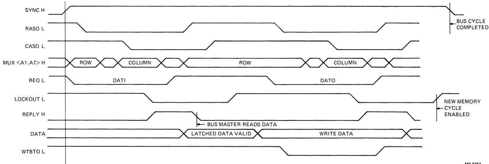
Figure A-4 DATIO(B) Signal Sequence
