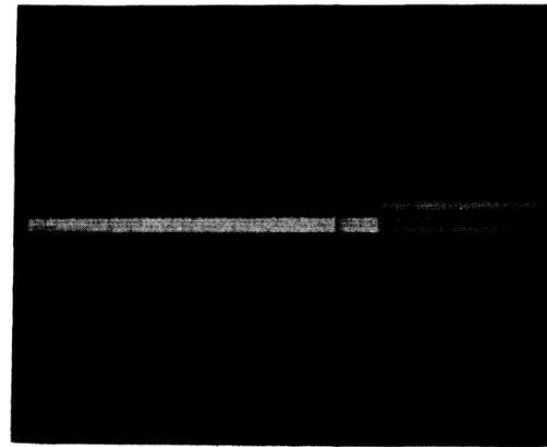
d. Head correctly aligned. Amplitudes are equal.
