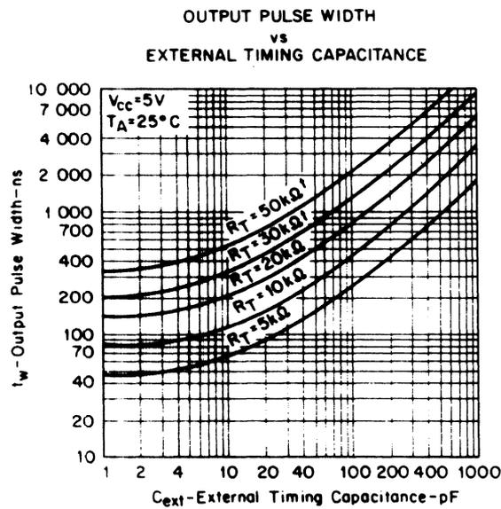
Figure A-3 DEC 74123 IC Output Pulse Width vs. External Timing Capacitance
