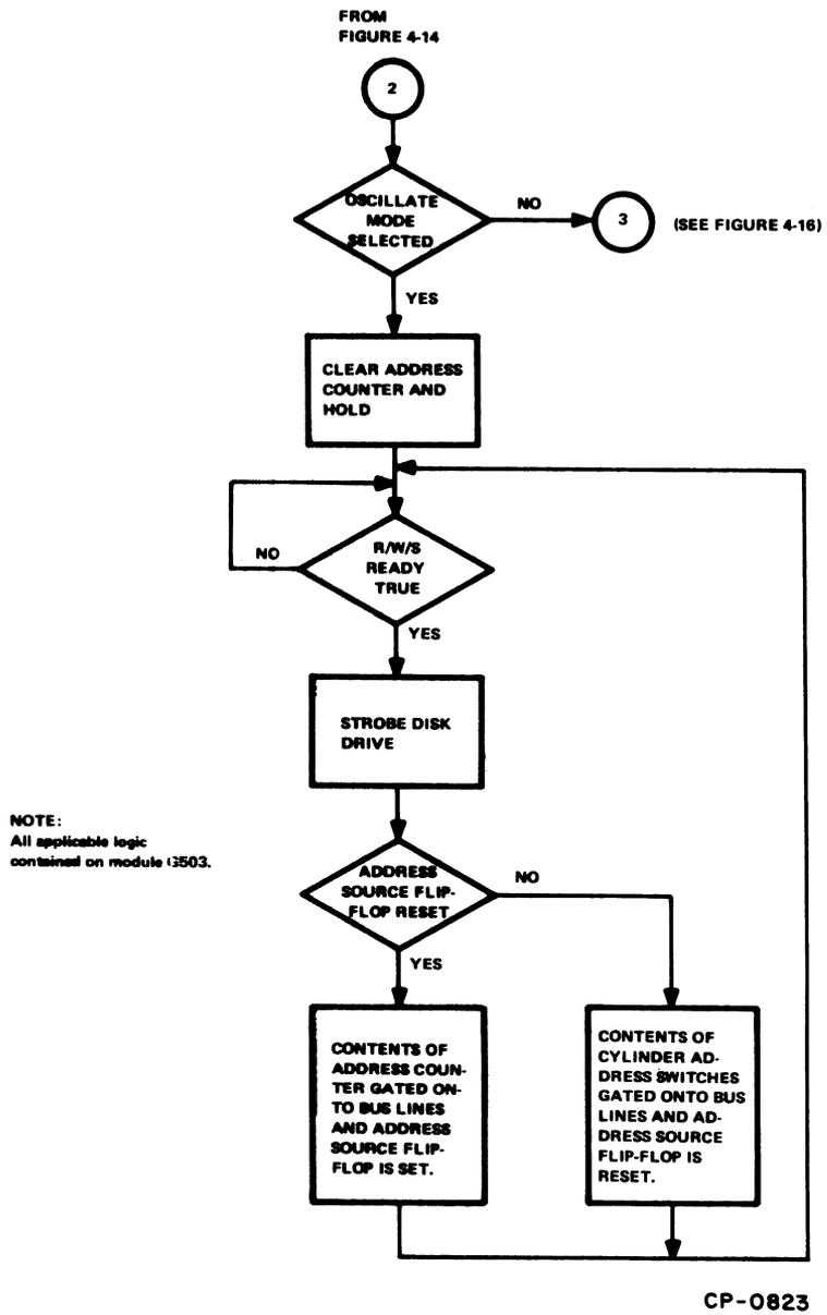
Figure 4-15 Positioner Exerciser Oscillate Mode Flow Diagram
