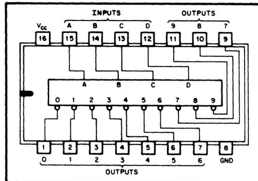
Figure A-1 7442 Package and Logic Diagrams
