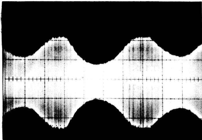
Figure 5-24 2315 CE Pack Head Alignment Waveforms (Sheet 1 of 3)
