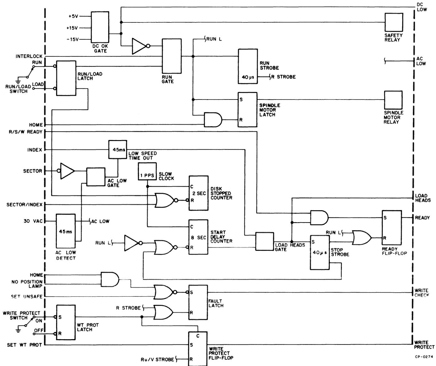
Figure 4-9 Control and Interlock Block Diagram
