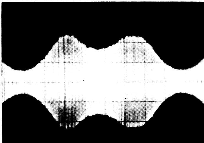
Figure 5-24 2315 CE Pack Head Alignment Waveforms (Sheet 2 of 3)
