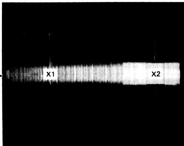
Figure 5-22 RK05K-AC Head Alignment Waveforms (Sheet 2 of 3)
