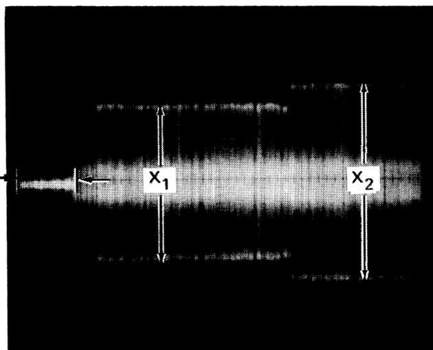
Figure 5-22 RK05K-AC Head Alignment Waveforms (Sheet 1 of 3)
