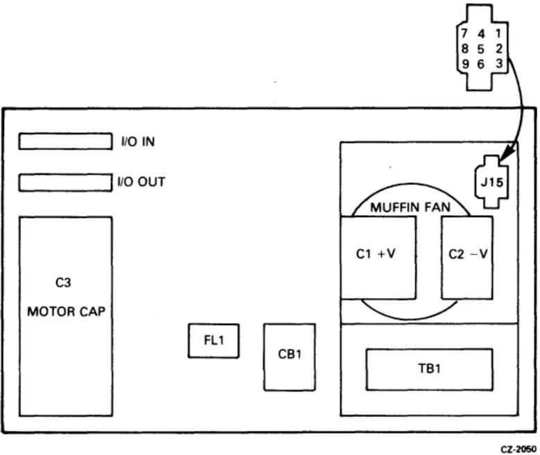
Figure 2-11 Power Panel Layout — Front View
