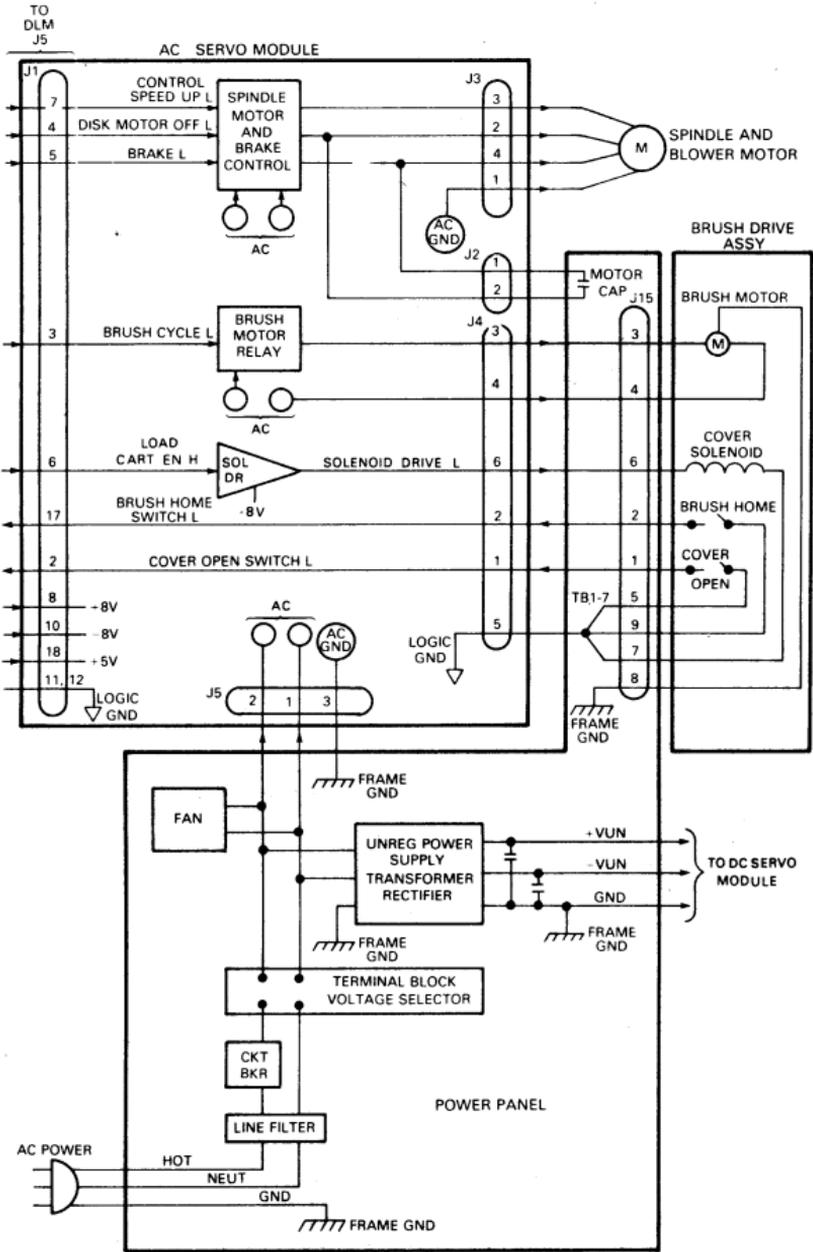
Figure 2-2 Signal and Function Diagram of Power Panel, AC Servo, Brush Drive Assembly
