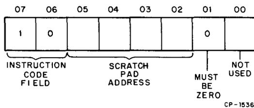
Some of the Scratch Pad memory locations are dedicated as fixed storage locations. For example, the first two locations store the current track address for units 0 and 1, respectively. Error and Status register information is also stored in fixed Scratch Pad locations. A breakdown of all Scratch Pad locations and their uses is given in the RX8/RX11 Print Sets.
