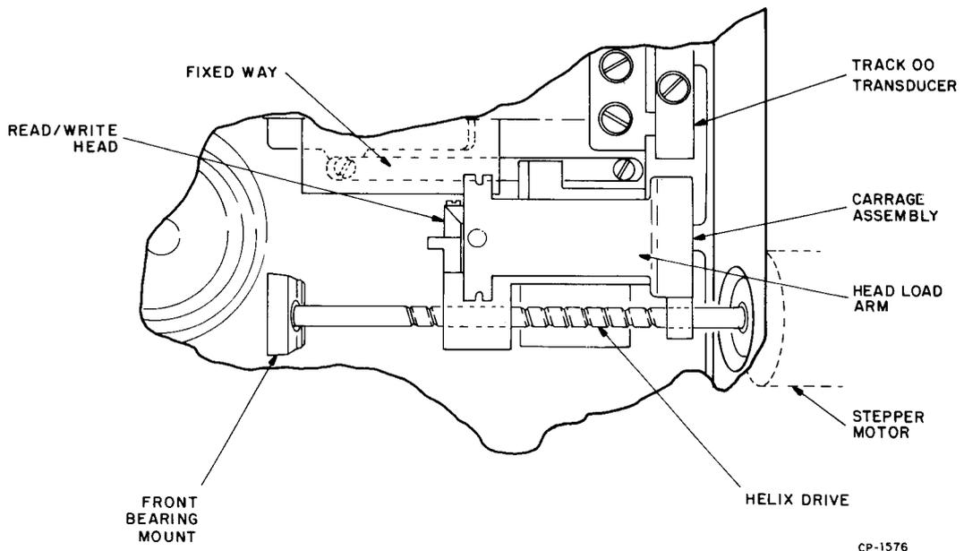
Figure 5-26 Positioning Mechanism
