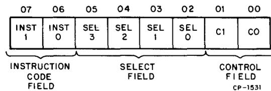
The high-order two bits of the control word are the instruction code bits, INST 0 and INST 1. There are five types of instructions, which are determined by these two bits and the C1 bit:
