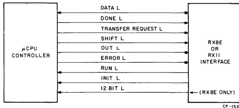
Figure 5-4 Interface to  $\mu$ CPU Controller Signals
