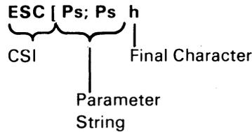
A control function is either a single character or a string of characters that affects the recording, processing, transmission, or representation of data. Control functions in the VT103 are classified in three ways, as follows.
