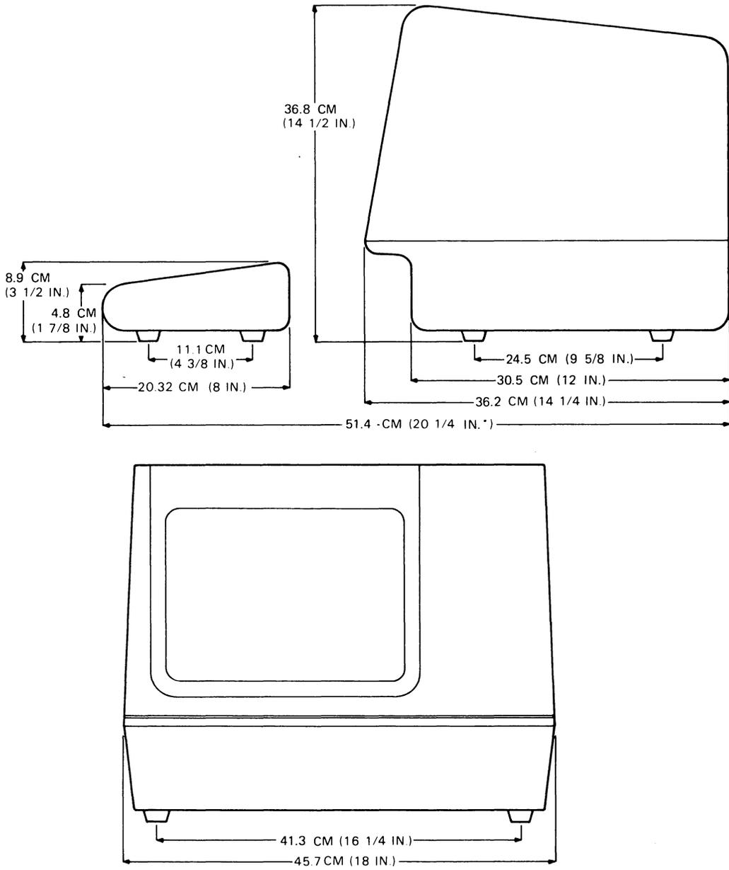
\* MEASUREMENT TAKEN WITH THE KEYBOARD PLACED FLUSH TO FRONT OF TERMINAL UNDER UNDERCUT.
