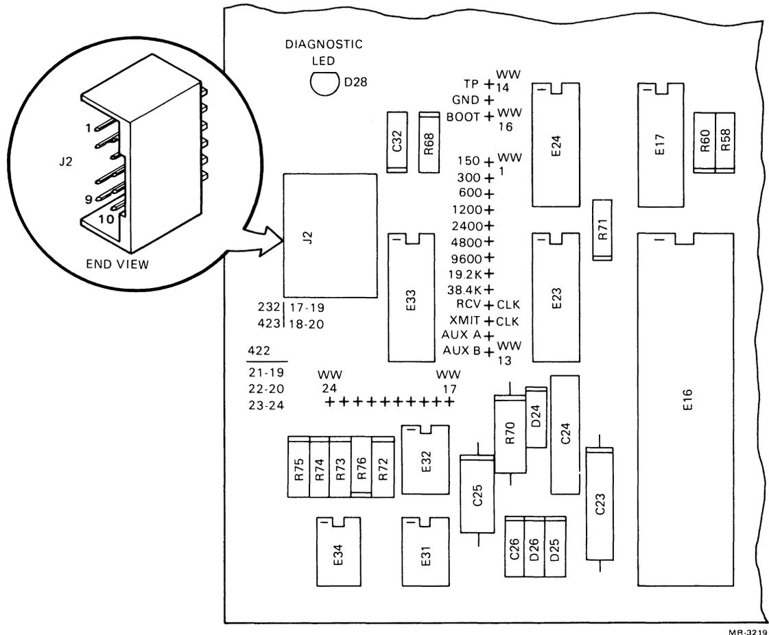
Figure 4-5 TU58 Controller Module Jumper Pin Locations
