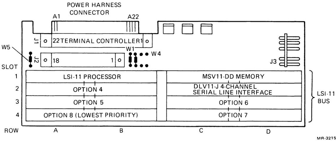
Figure 3-5 Example 1: Configuring the LSI-11 Bus
