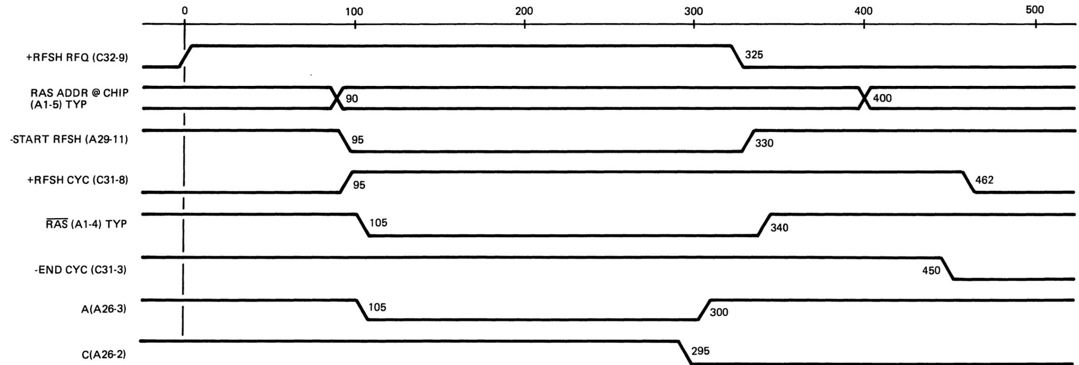
Figure 2-4. Internal Timing Sequence Refresh Cycle
