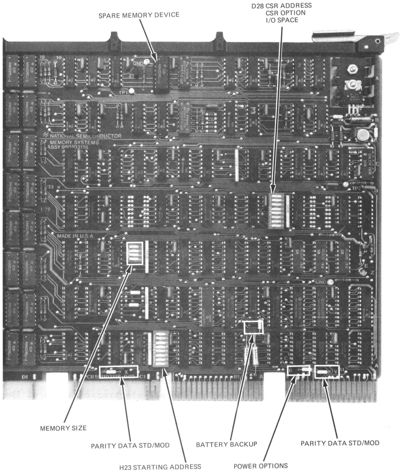
Figure 3-1. Jumper and Switch Locator
