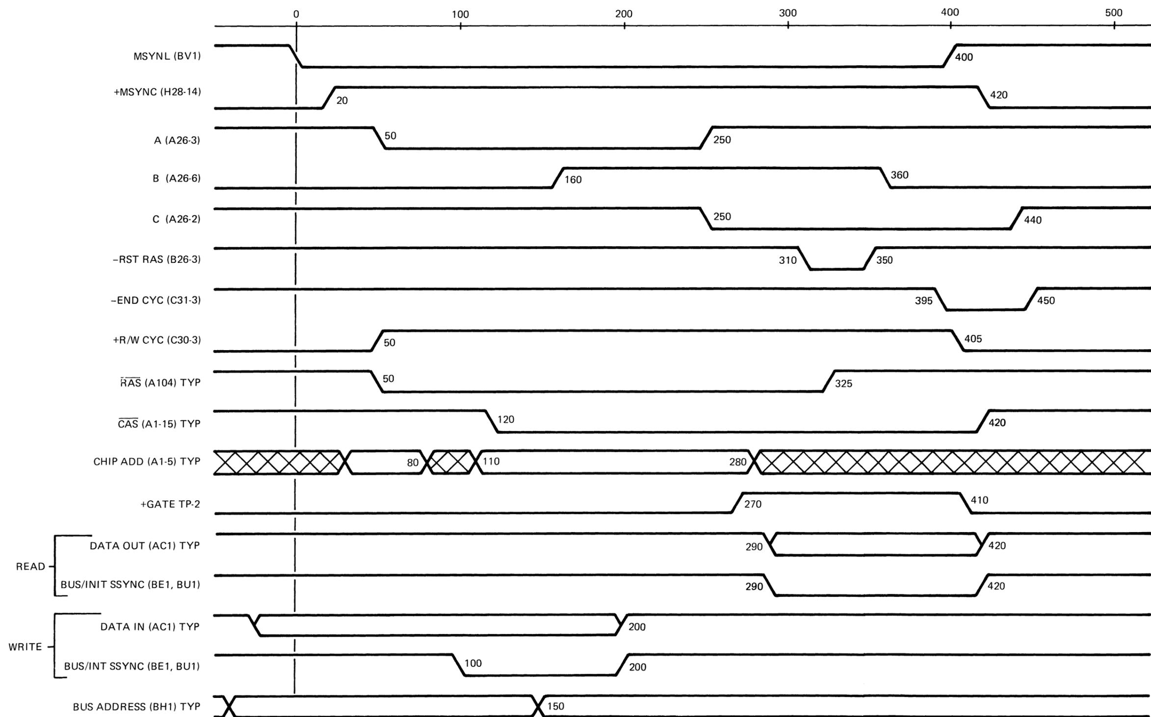
Figure 2-3. Internal Timing Sequence Read and Write Cycles
