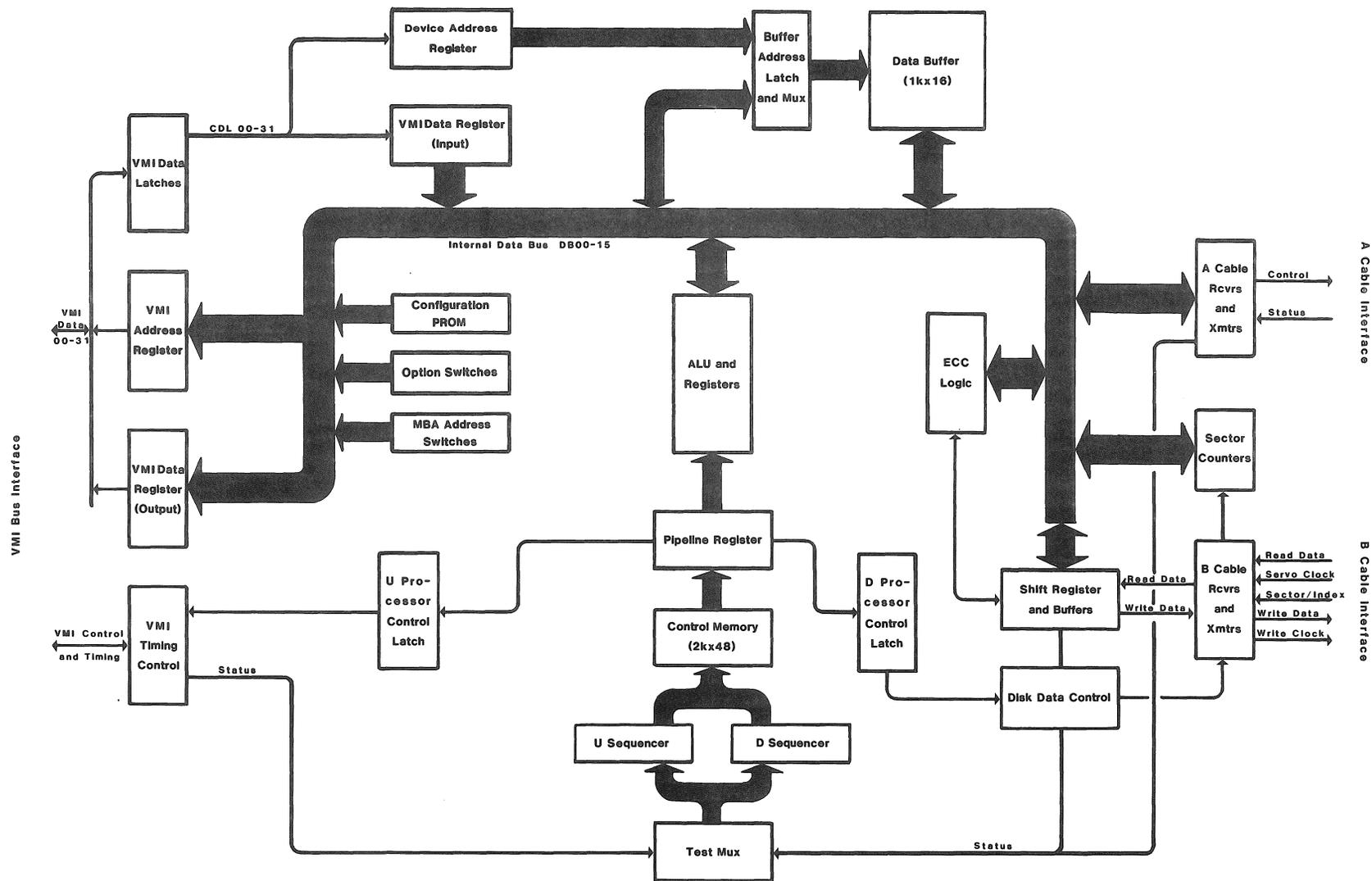
Figure 2-2. SC780 Block Diagram
