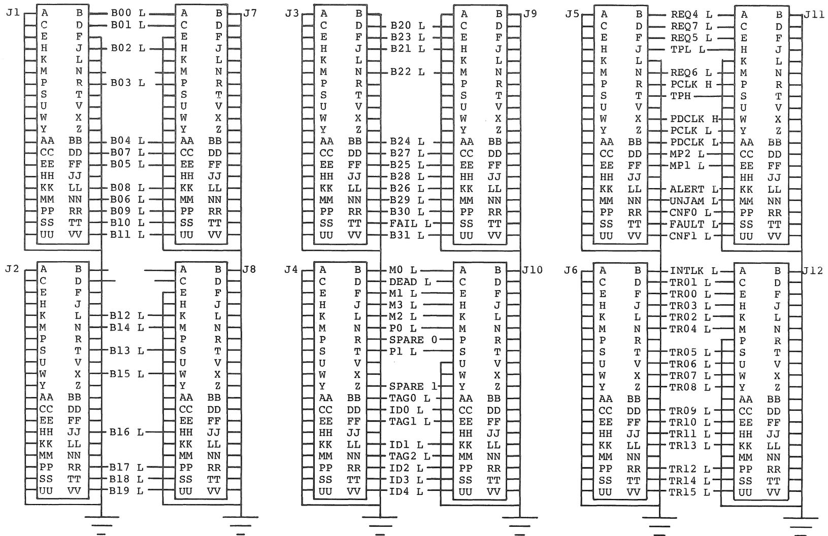
Figure 2-4. SBI Signal Names and Pin Assignments
