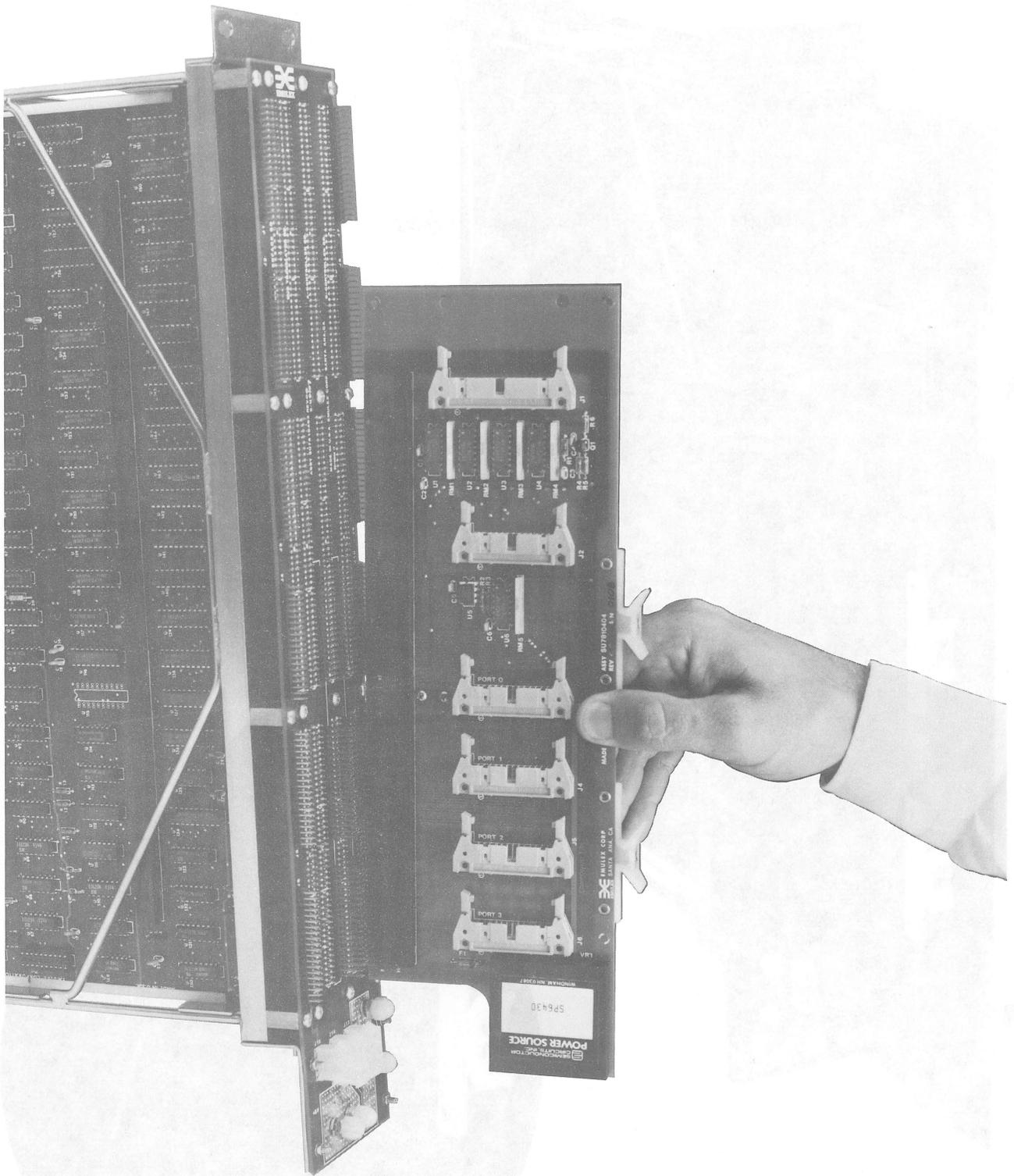
**Figure 3-7 Paddle Board Installation**
