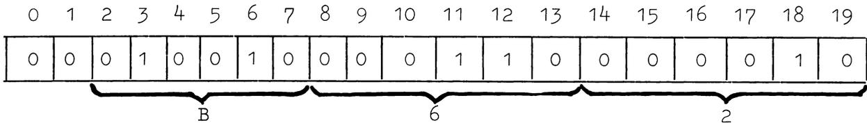
Bit positions 2 to 19 store the three six-bit binary coded decimal digits, while bit positions 0 and 1 may be used to hold other information.
