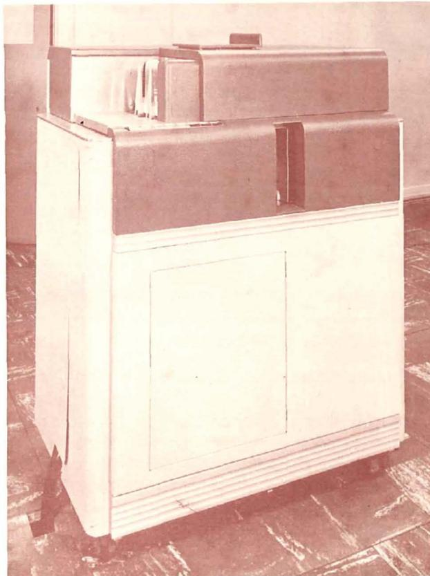
The card punch equipment can punch cards in the two formats described in the previous section on the card reading equipment. Data re-arrangement can be achieved through program and/or card punch plugboard control.
