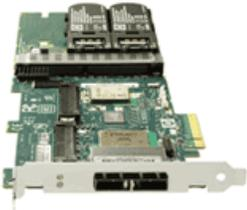
The HP Smart Array P800 is a 16 port, PCI-Express SAS controller. It ships standard with 512MB cache, dual batteries, and RAID 6 (ADG) support. This controller supports up to 108 hard drives and is the highest performing controller in the Smart Array portfolio.
