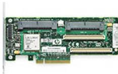
The HP Smart Array P400i is the integrated version of the P400, HP's first PCI-Express (PCI-Express) serial attached SCSI (SAS) RAID controller, that provides new levels of performance and reliability for HP servers through its support of the latest SCSI technology and advanced RAID capabilities.
