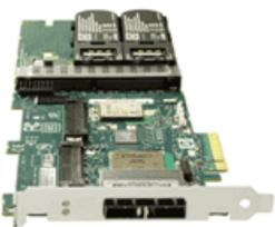
The HP Smart Array P800 is a 16 port, PCI-Express SAS controller. It ships standard with 512MB cache, dual batteries, and RAID 6 (ADG) support. This controller supports up to 108 hard drives and is the highest performing controller in the Smart Array portfolio.
