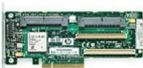
The HP Smart Array P400 is HP's first PCI-Express (PCIe) serial attached SCSI (SAS) RAID controller and provides new levels of performance and reliability for HP servers, through its support of the latest SCSI technology and advanced RAID capabilities.
