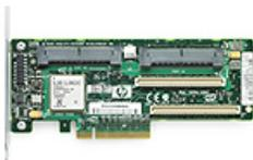
The HP Smart Array P400i, used in this benchmark, is HP's first PCI-E SAS RAID controller and provides new levels of performance and reliability for HP servers through its support of the latest SCSI technology and advanced RAID capabilities. The Smart Array P400i is ideal for SAS-based servers and storage enclosures that require mission-critical reliability and high performance.
