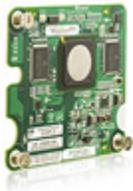
The QLogic QMH2462 4Gb FC HBA Adapter provides the c-Class BladeSystem with two 4Gb Fibre Channel ports for fast and reliable SAN connectivity. Through the implementation of a SAN with the HP BladeSystem, customers can achieve improved data availability, easily scale capacity, and realize management cost savings from consolidating disk resources.
