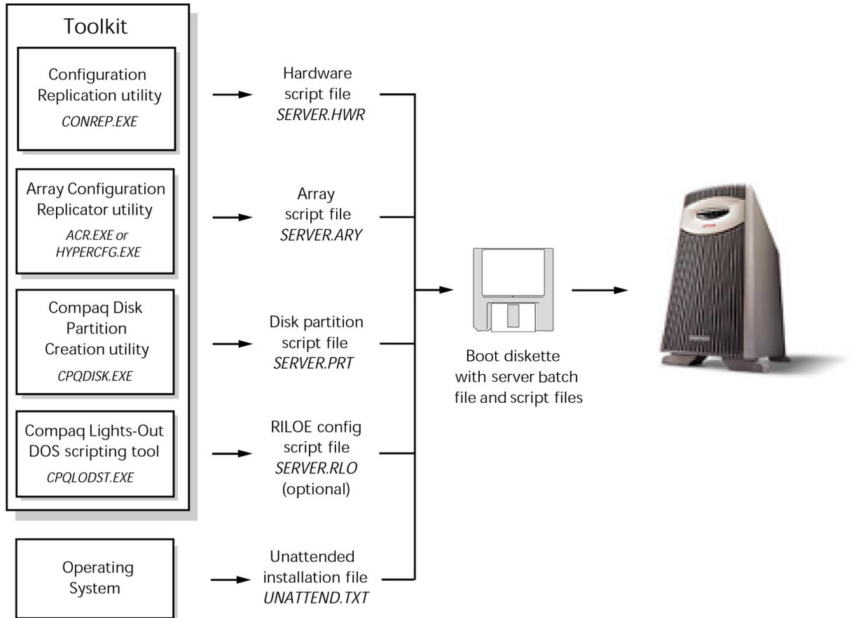
**Figure 1-1: SmartStart Scripting Toolkit server deployment process**
