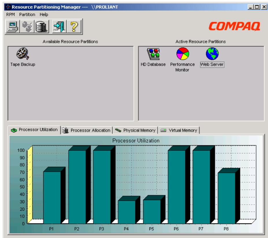
Figure 2. The RPM GUI includes windows for available resource partitions, active resource partitions, and real-time processor and memory utilization.
