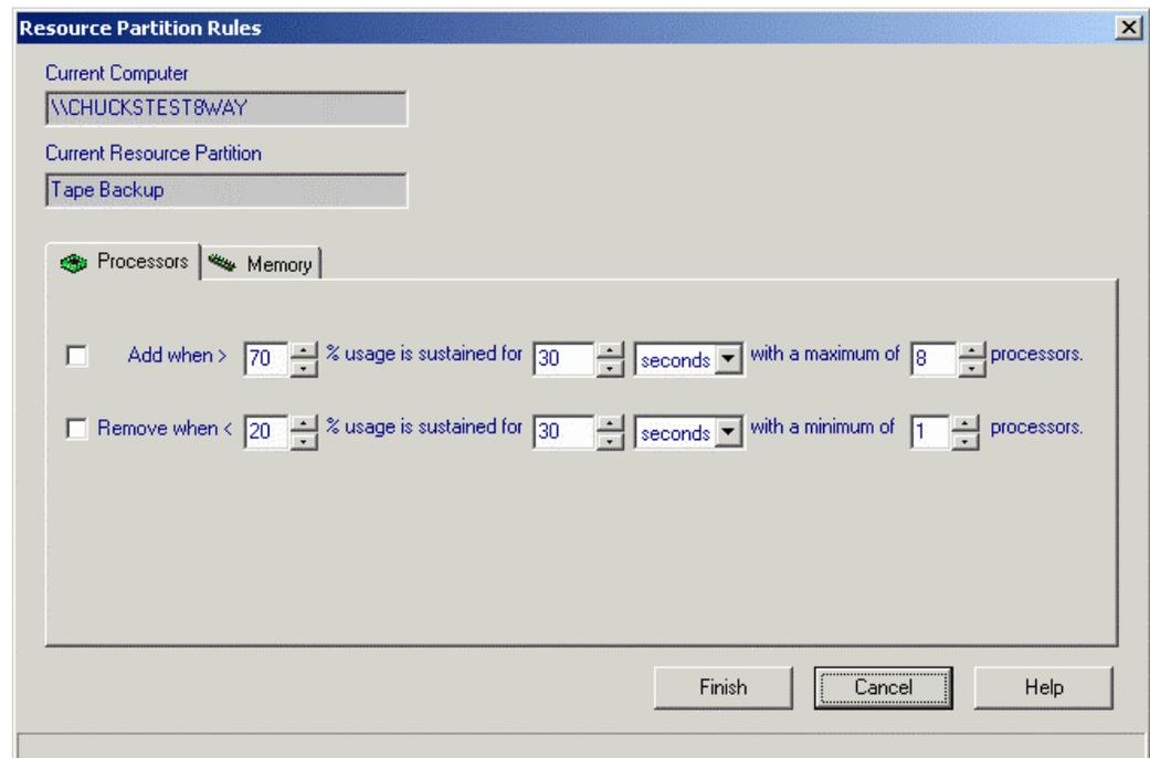
Figure 3. The RPM GUI leads the administrator through choices to establish rules for the processor and memory allocation.
