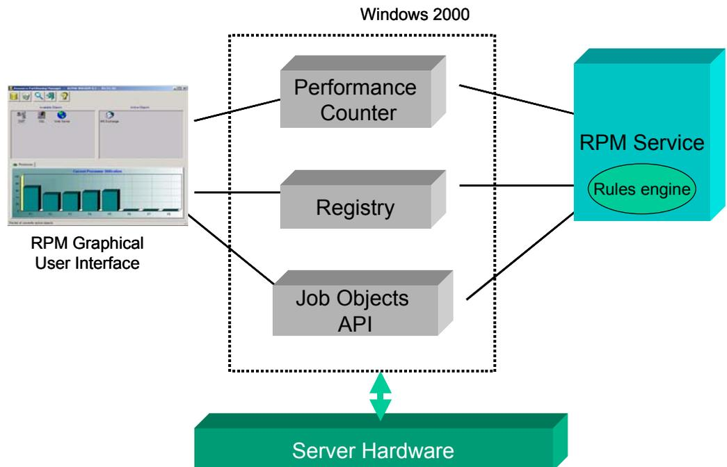
Figure 1. RPM architectural diagram
