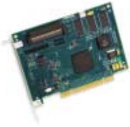
This low-cost, single-channel SCSI controller is designed for entry-level and workgroup servers.
