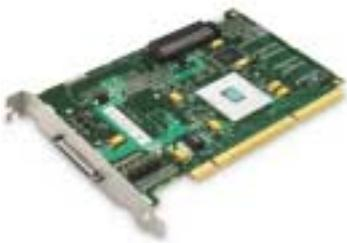
The Smart Array 532 Controller delivers exceptional value for entry-level and workgroup servers, without sacrificing performance. This controller features two Ultra3 SCSI channels, allowing for the configuration of up to 28 hard drives to store up to 2TB of storage per server PCI slot.
