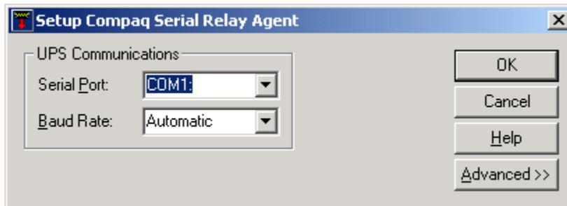
A message is displayed asking to start the Serial Relay Agent. Click **Yes**. The installation program attempts to communicate with the UPS. After communication is established, the **Service Start** screen is displayed.
