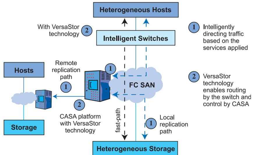
Figure 2. CASA and Switches with VersaStor Technology
