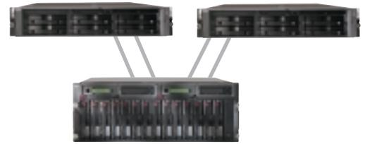
MSA500 G2 connected to two HP ProLiant DL380 servers via SCSI with multi-path I/O option
