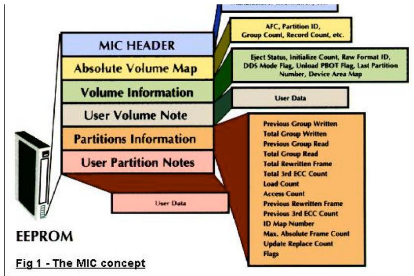
The information stored within the MIC consists of a combination of drive and user generated information, as shown in the illustration. The user information is accessible using two Vendor Unique SCSI commands, called "AIT MIC Select" and "AIT MIC Sense." Drive-related information is stored and retrieved automatically under the control of the drive firmware.
