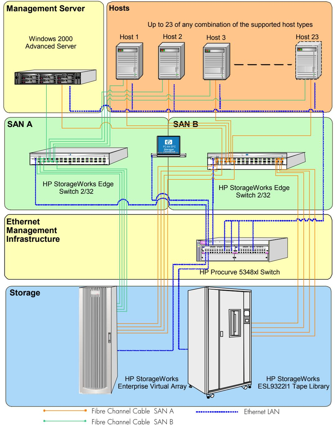
**figure 2. example mid-tier consolidation solution: physical view**
