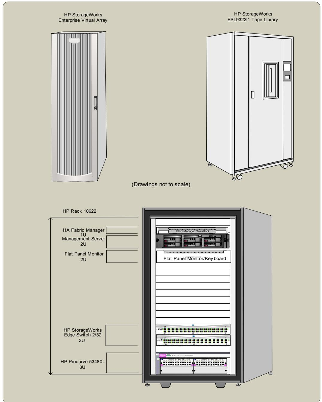
**figure 3. example mid-tier consolidation solution rack**
