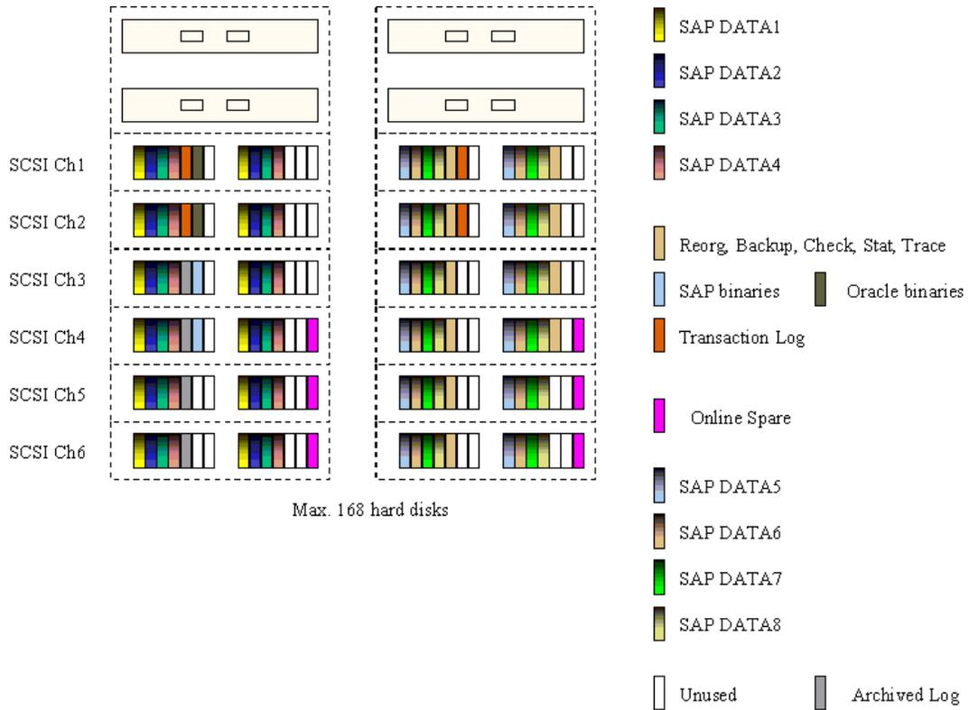
Figure 7, StorageWorks EMA12000 - Oracle High-end Capacity
