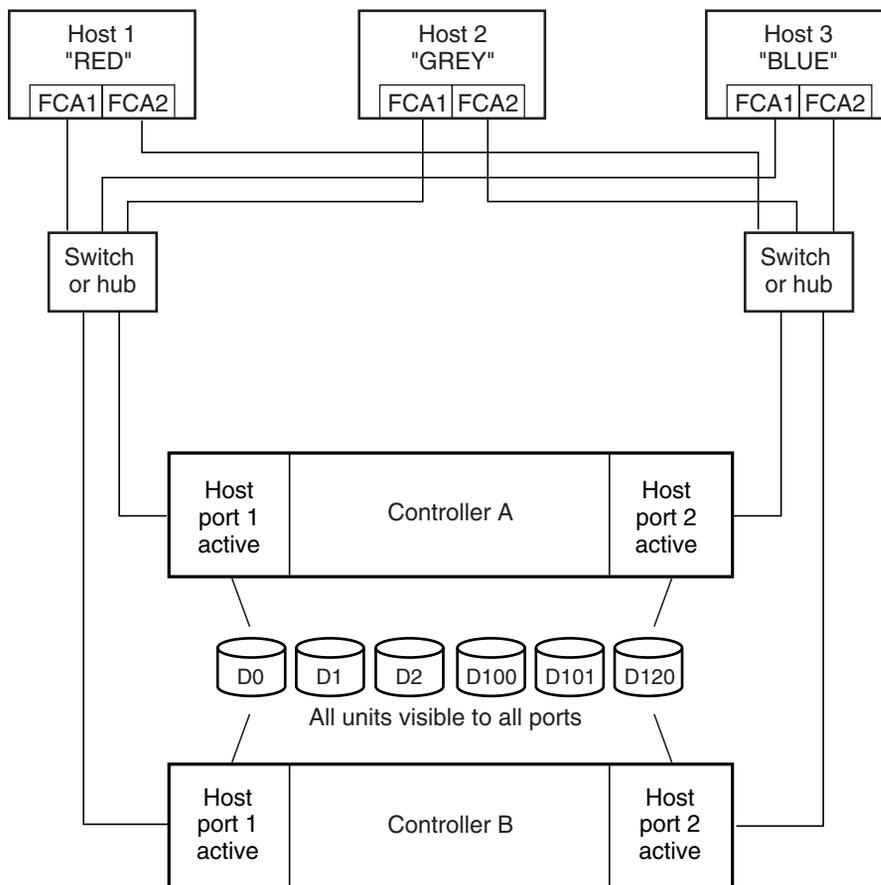
NOTE: FCA = Fibre Channel Adapter
