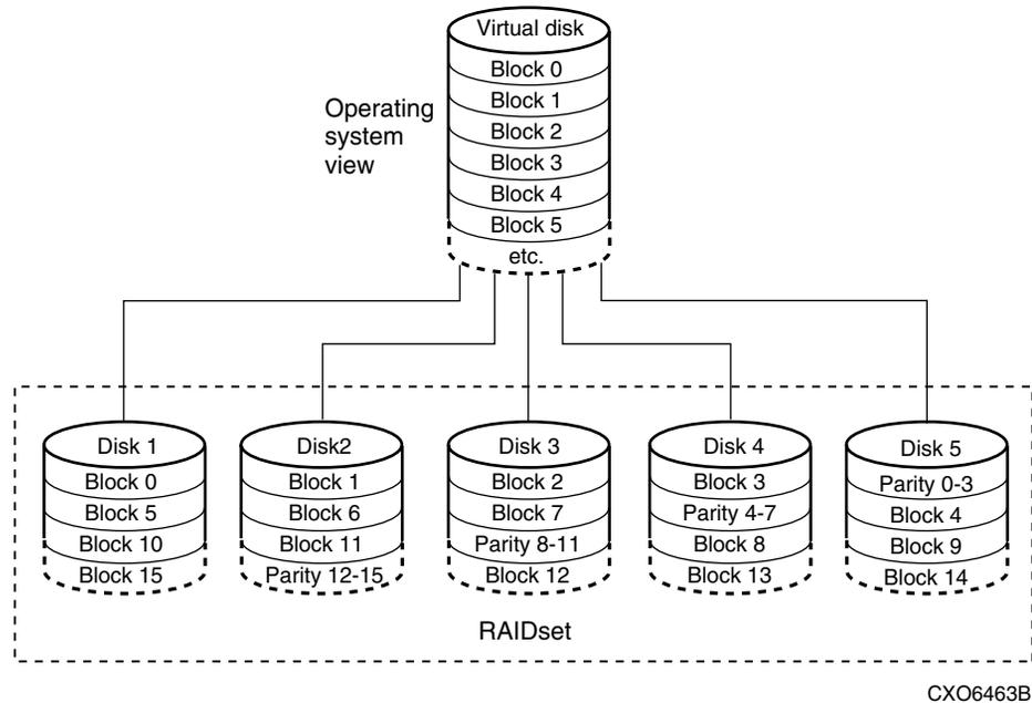
**Figure 2–9: 5-member RAIDset using parity**
