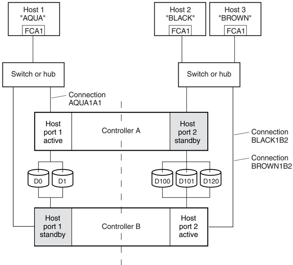
NOTE: FCA = Fibre Channel Adapter
