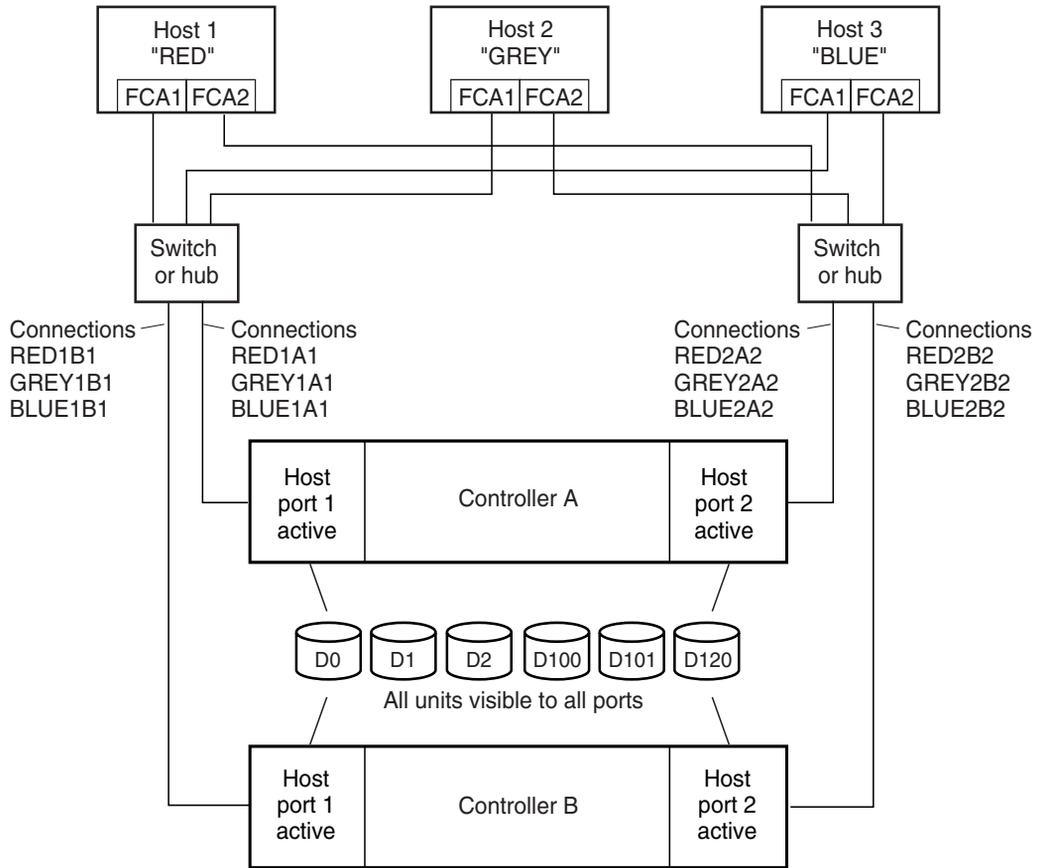
NOTE: FCA = Fibre Channel Adapter
