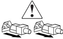
Power Supplies or Systems marked with these symbols indicate that the equipment is supplied by multiple sources of power.
