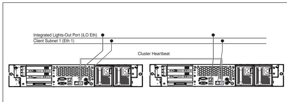
**Figure 4: NAS b3000 v2 cluster deployment**
