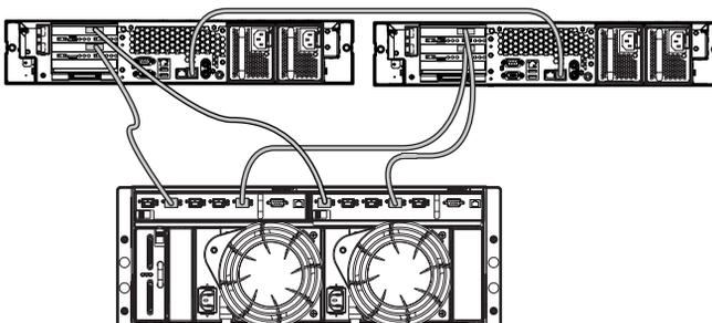
**Figure 2: NAS b3000 v2 as a clustered pair of devices**
