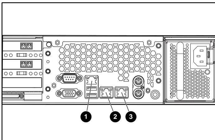
**Figure 6: Ethernet connectors**
