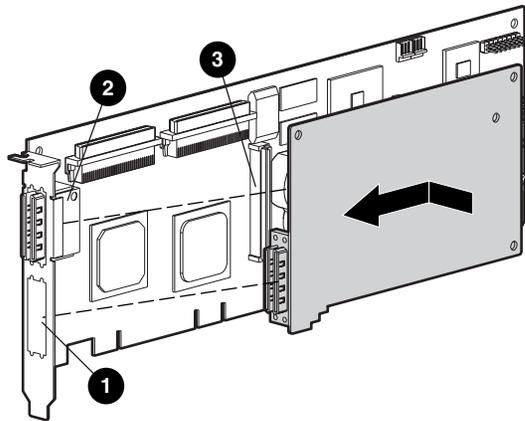
2. Plug the adapter board into the connector ❸ on the array controller board.
