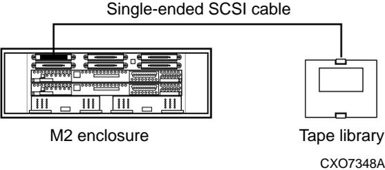
Figure 8-11. MA8000 and EMA12000 (Modula) Tape Device Cabling - Configuration 1
