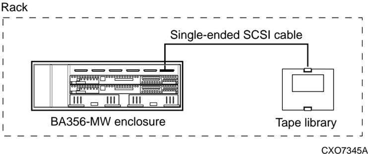
Figure 8-8. SW800 and SW500 Tape Device Cabling - Configuration 2
