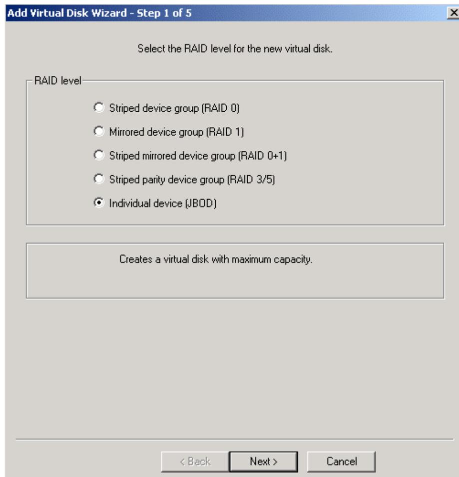
Figure 5-19. Adding Virtual Disk Wizard (Step 1 of 5)
