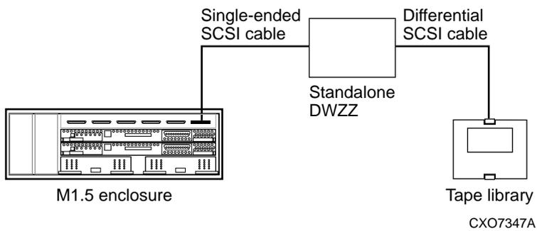
Figure 8-10. SW800 and SW500 Tape Device Cabling - Configuration 4
