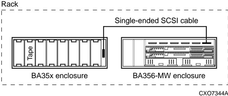
Figure 8-7. SW800 and SW500 Tape Device Cabling - Configuration 1
