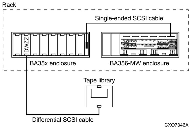
Figure 8-9. SW800 and SW500 Tape Device Cabling - Configuration 3
