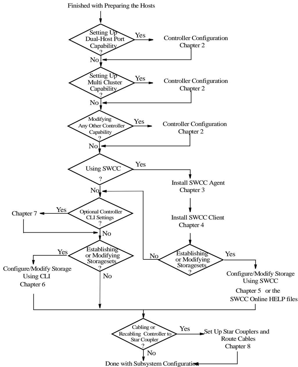
Figure 1-1. Configuration Flow
