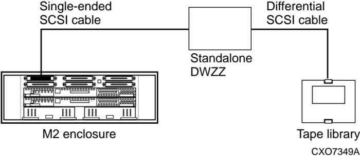
Figure 8-12. MA8000 and EMA12000 (Modula) Tape Device Cabling - Configuration 2
