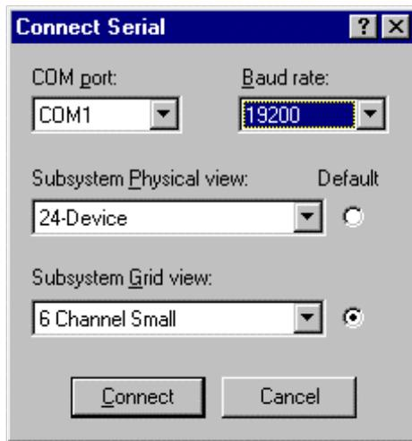
Figure 5-3. Connect Serial Dialog Box for Storage Window
