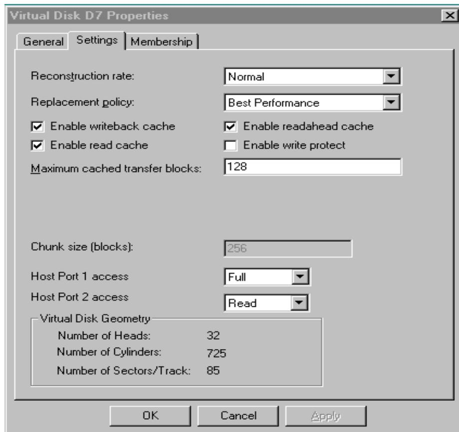
Figure 5-26. Virtual Disk Properties Settings Tab
