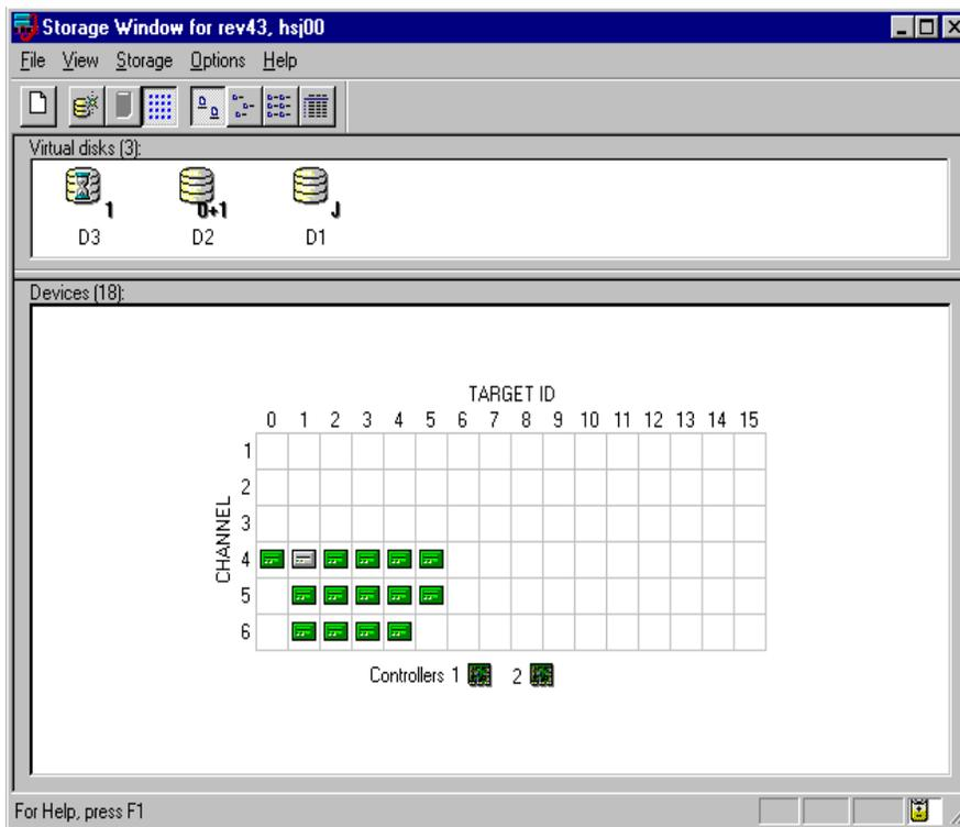
Figure 5-24. Storage Window During Creation Of Virtual Disks (D3)
