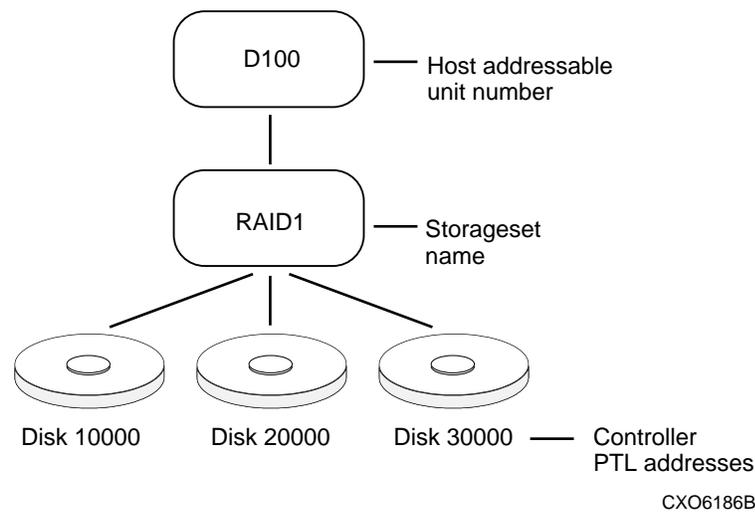
Figure 2-3. Mapping a Unit to Physical Disk Drives
