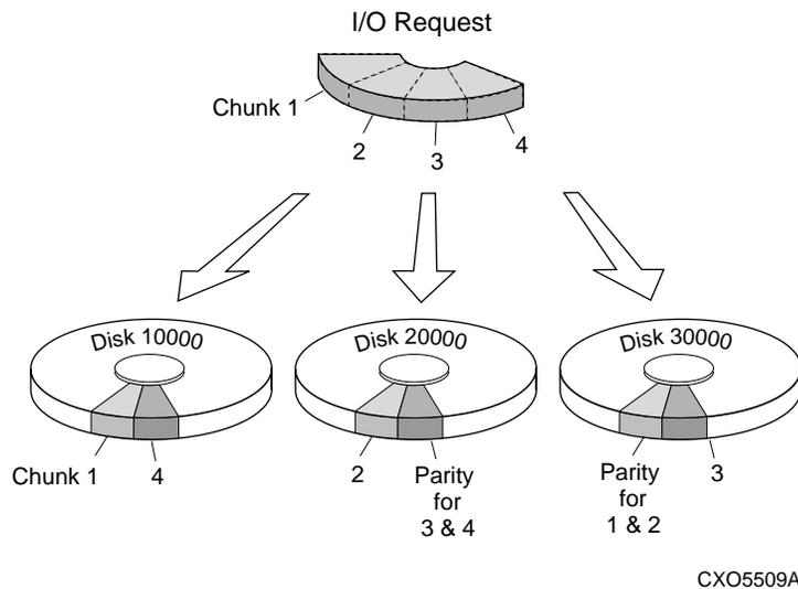
Figure 2-12. Three-Member RAIDset Using Parity (Example 1)
