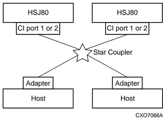
Figure 1-4. Dual Controller, Single Host Port, Single Cluster Configuration
