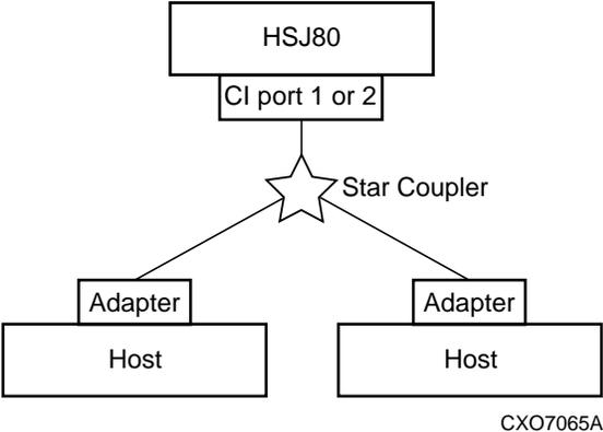
Figure 1-3. Single Controller, Single Host Port, Single Cluster Configuration
