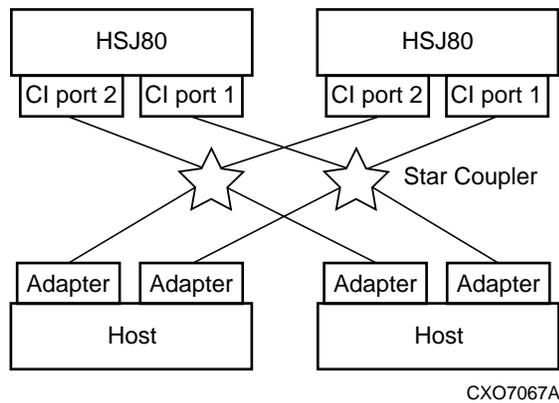
Figure 1-5. Dual Controller, Dual Host Port, Dual Star Coupler Configuration
