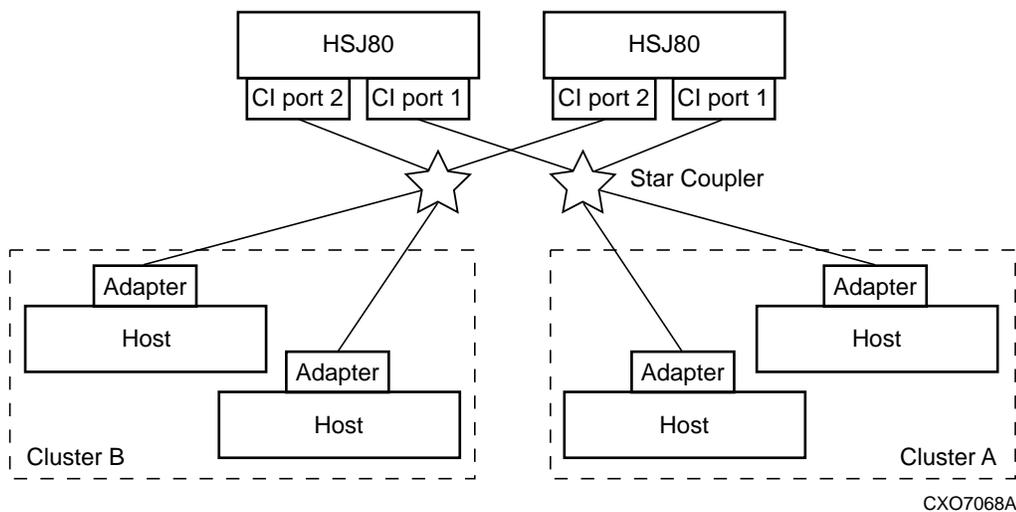
Figure 1-6. Dual Controller, Dual Host Port, Multiple-Cluster Configuration
