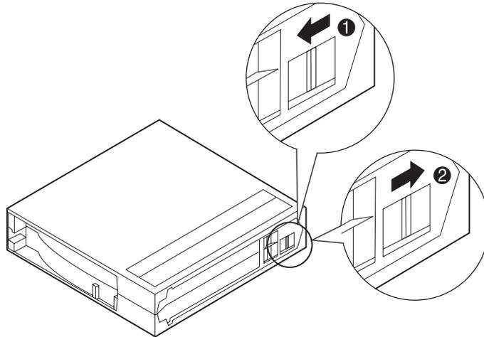
Figure 15: Cartridge write-protect switch
