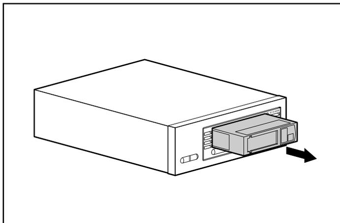
**Figure 14: Removing a DLTape IV cartridge**
