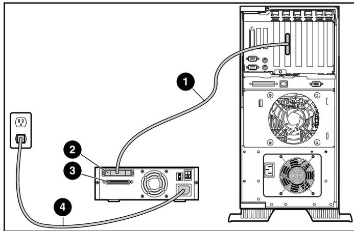
**Figure 4: Connecting a single external drive**
