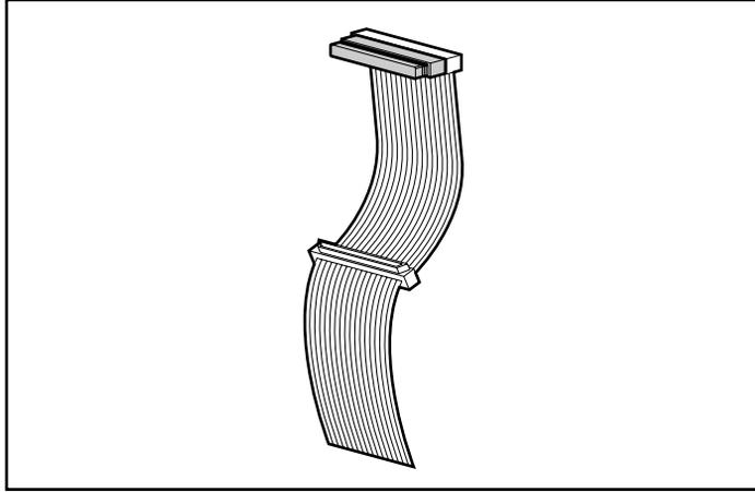
Figure 9: Ribbon cable with terminator
