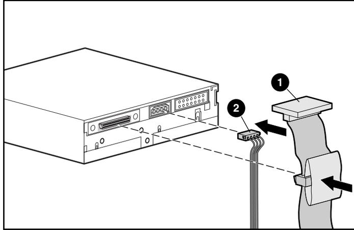
**Figure 11: Connecting the power and signal cable**
