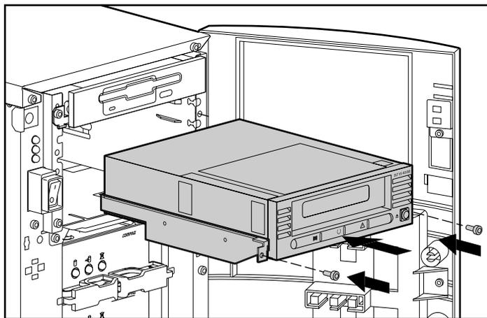
**Figure 10: Installing an internal drive**
