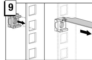
Insert the cage nuts into the rack rails and use the fitting tool to pry the cage nut into position.
