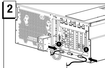
Connect the mouse 1 and the external keyboard 2 to the "Y" cable (optional).
