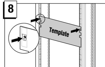
Mark the front and back of the rack using the server rack template.
