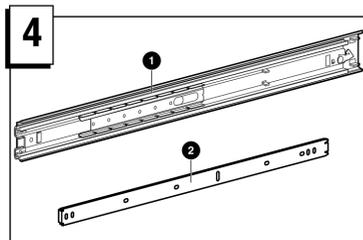
Separate the outer bracket rail 1 and server rail 2.
