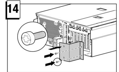
Secure the cable management arm server bracket to the StorageWorks NAS Executor E7000.
