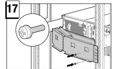
Attach the cable management arm to the rear brace of the rack.
