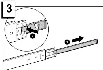
a. Extend the server rail from the outer bracket rail until the server rail release latch clicks.
