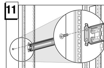
Secure the front of the rack mounting bracket to the rack using M6 x 12 mm Phillips head screws.
