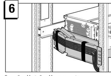
Secure the cables to the cable management arm.
