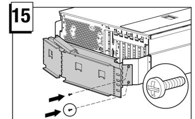
Secure the cable management arm to the cable management server bracket using two screws.
