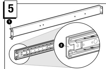
Identify the outer bracket rail 1 and the front of the rack-mounting bracket 2.
