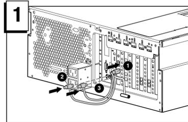
Connect the keyboard/mouse "Y" cable 1 to the Remote Insight Lights-Out Edition board and to the server mouse connection 2 and keyboard connection 3.
