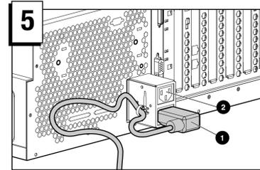
Connect the power cords to the primary 1 and secondary 2 power cord connectors.
