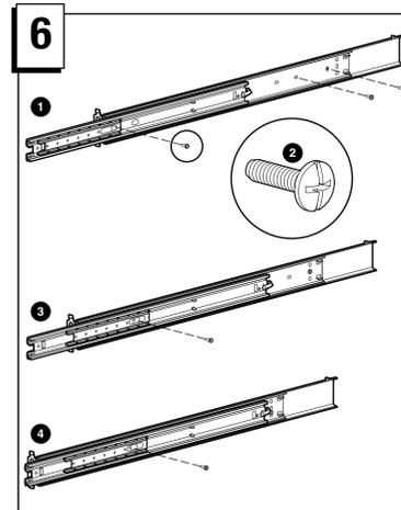
a. Fully extend the inner slide from the front of the outer bracket rail 1.
