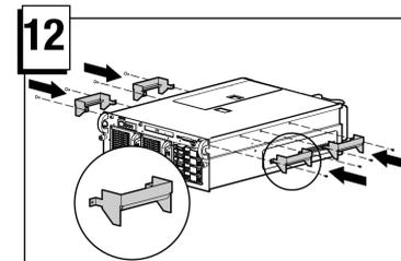
Attach the handle to the sides of the NAS Executor E7000.
