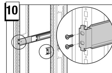
Secure the back of the rack mounting bracket to the rack using M6 x 12 mm Phillips head screws.
