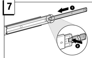
Replace the server rail by aligning it with the front mounting bracket and sliding forward until you hear a click 1. Press the latch in 2 and slide the server rail through the jacket assembly until it stops.
