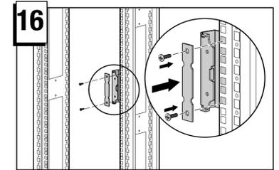
Attach the cable management arm screw-retaining plate.
